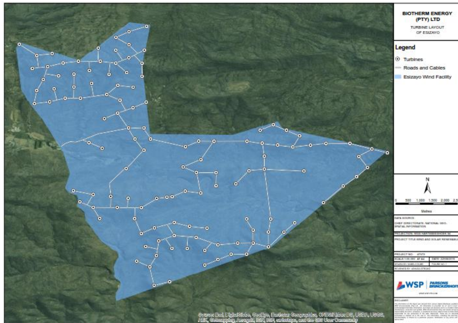
Esizayo Initial Turbine Layout (125 Turbines – 250 MW)
