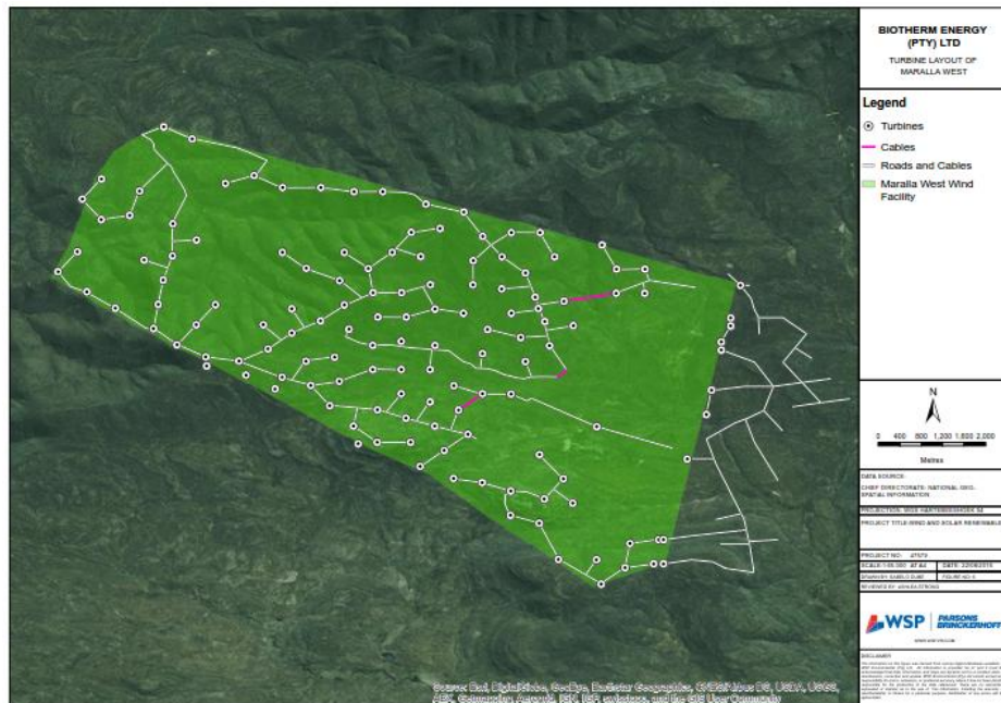
Maralla West Initial Turbine Layout (125 Turbines – 250 MW)
