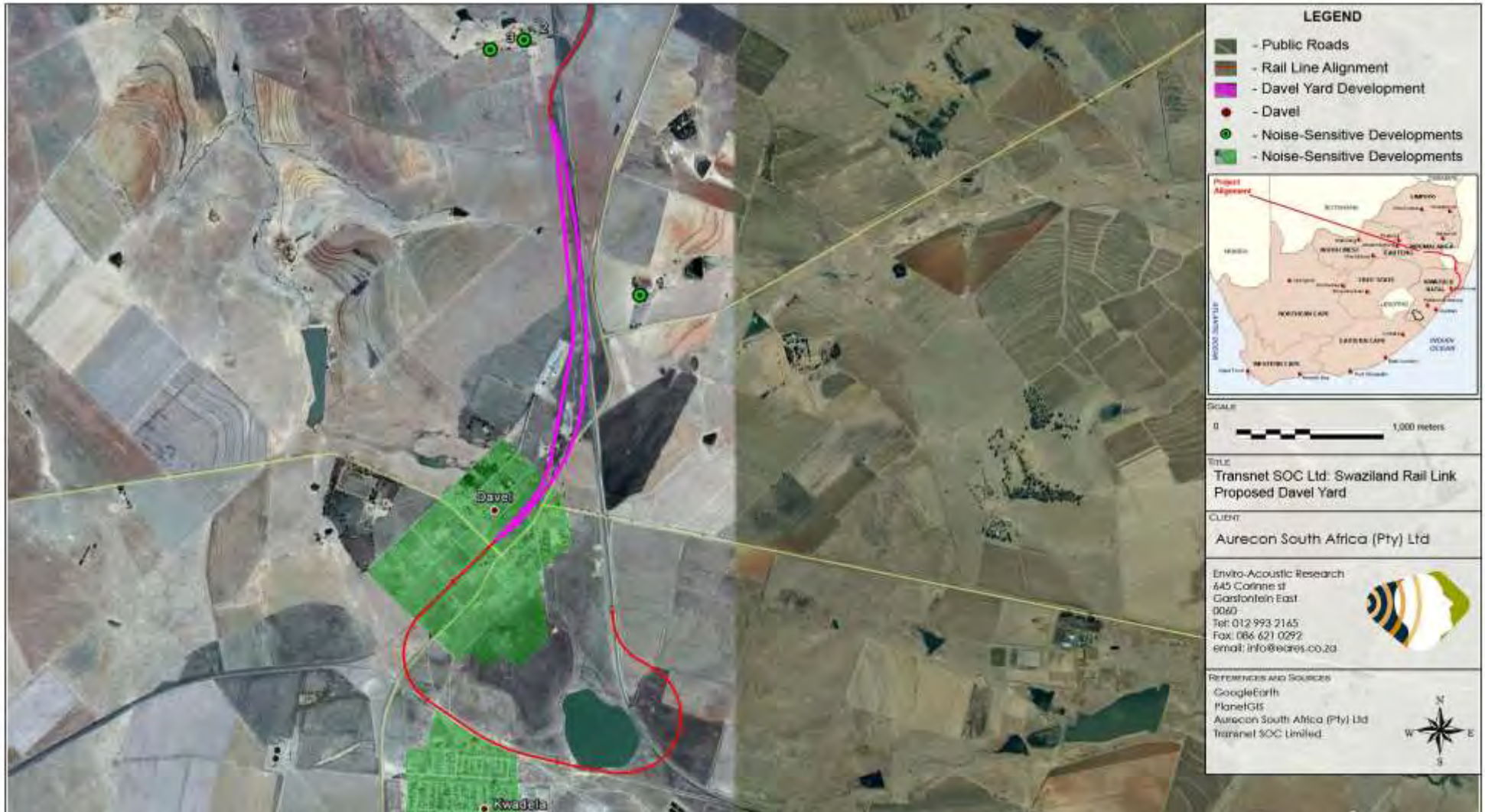
Figure 6: Noise sensitive receptors for the receiving environment
