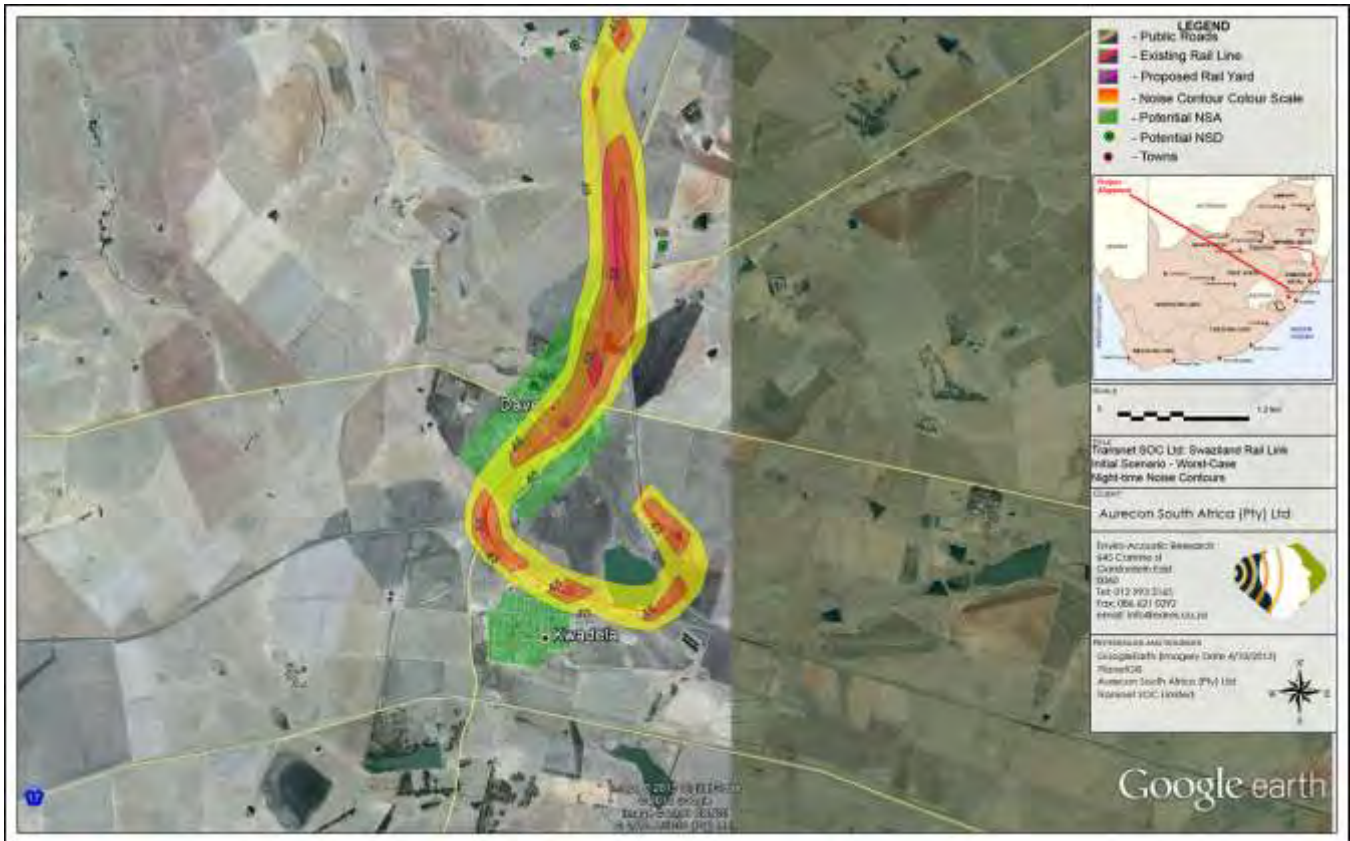
Figure 36: Projected initial scenario – Modelled worst-case night-time noise levels (no 12 dBA highly impulsive correction – shunting)
