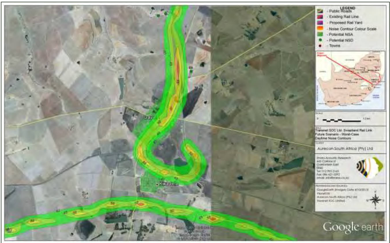
Figure 37: Projected future scenario – Modelled worst-case daytime noise levels (no 12 dBA highly impulsive correction – shunting)
