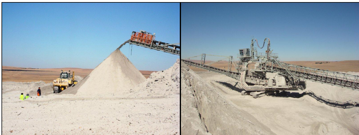
Figure 10.1: Stacker being used to dispose of ash at the Majuba power station
