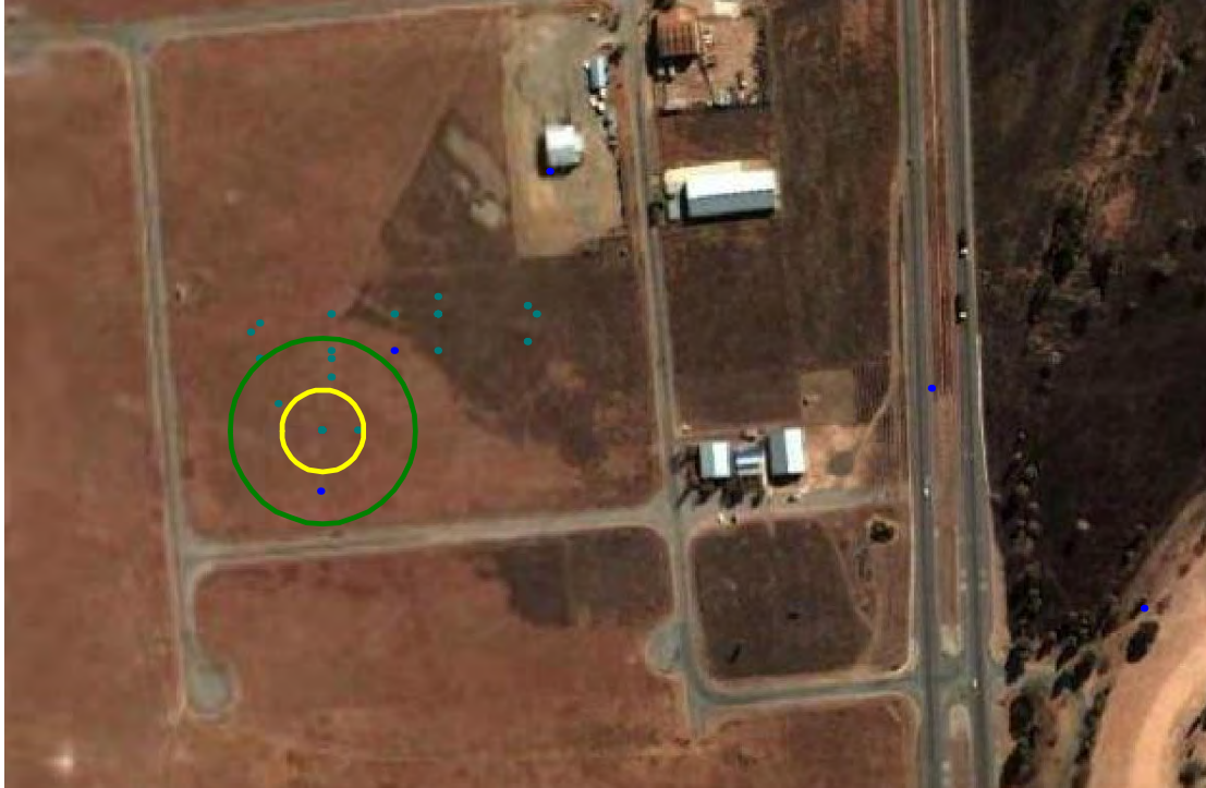
Radiation circles from the fire-balling of the reboiler on the distillation plant (Note the yellow line is the MHI threshold)
