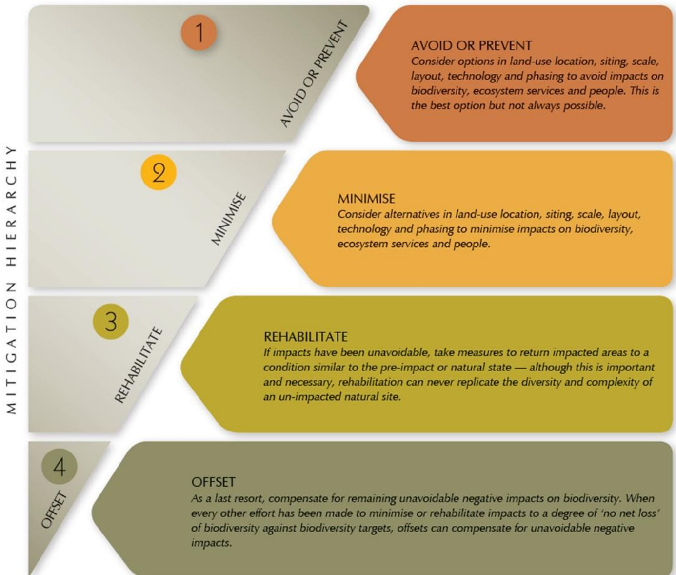
Figure 13: The Mitigation Hierarchy consists of 4 steps: avoid and prevent, minimise, rehabilitate and offset.
