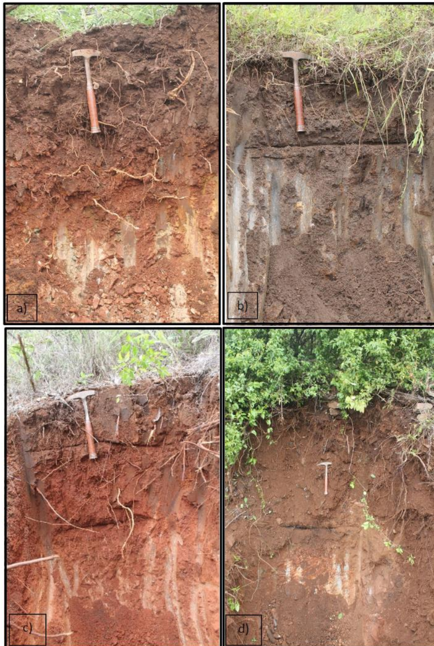
FIGURE 13: PHOTOGRAPHS OF SELECTED SOIL TYPES FOUND IN THE DIFFERENT STUDY AREAS; A-SWARTLAND SOIL FORM WITH A DARK ORTHIC HORIZON AND SAPROLITHIC C-HORIZON; B- SHALLOW WASBANK SOIL FORM WITH A HARD PLINTHIC C-HORIZON; C- A DEEP HUTTON WITH A LUVIC RED APEDAL SUBSOIL; D- A NCONKONI SOIL FORM.
