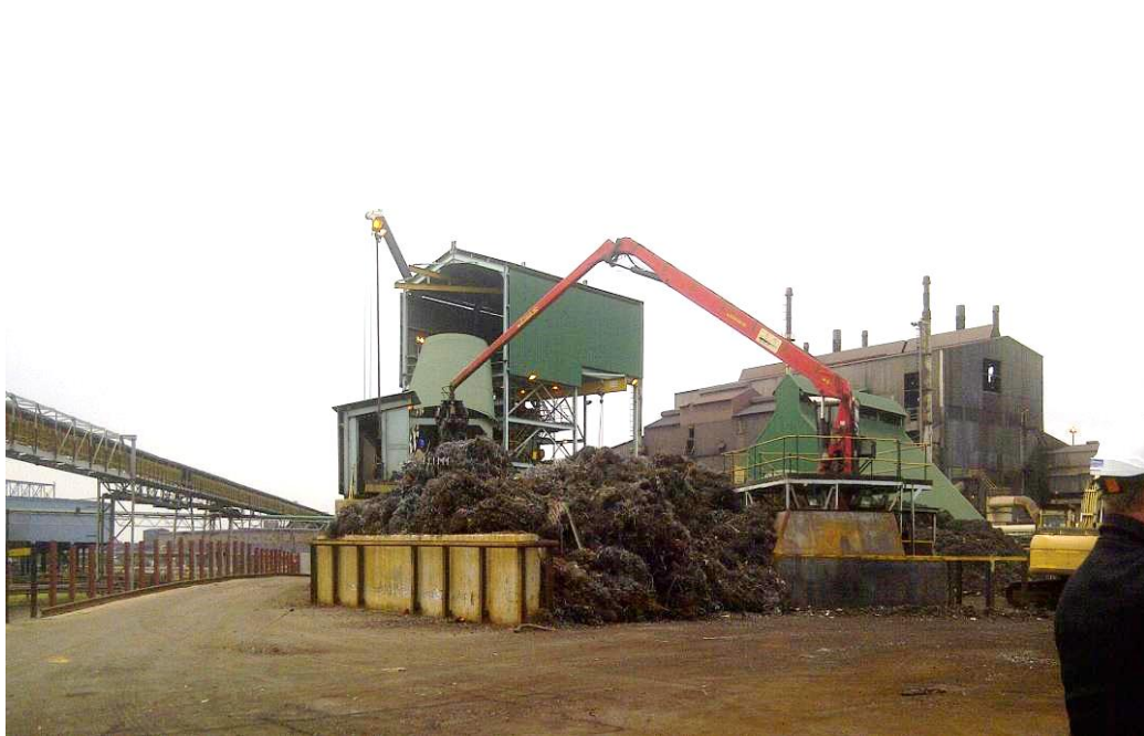
Figure 5: Steel shaving stockpile area showing magnet that loads the shavings onto feeding vibrators
