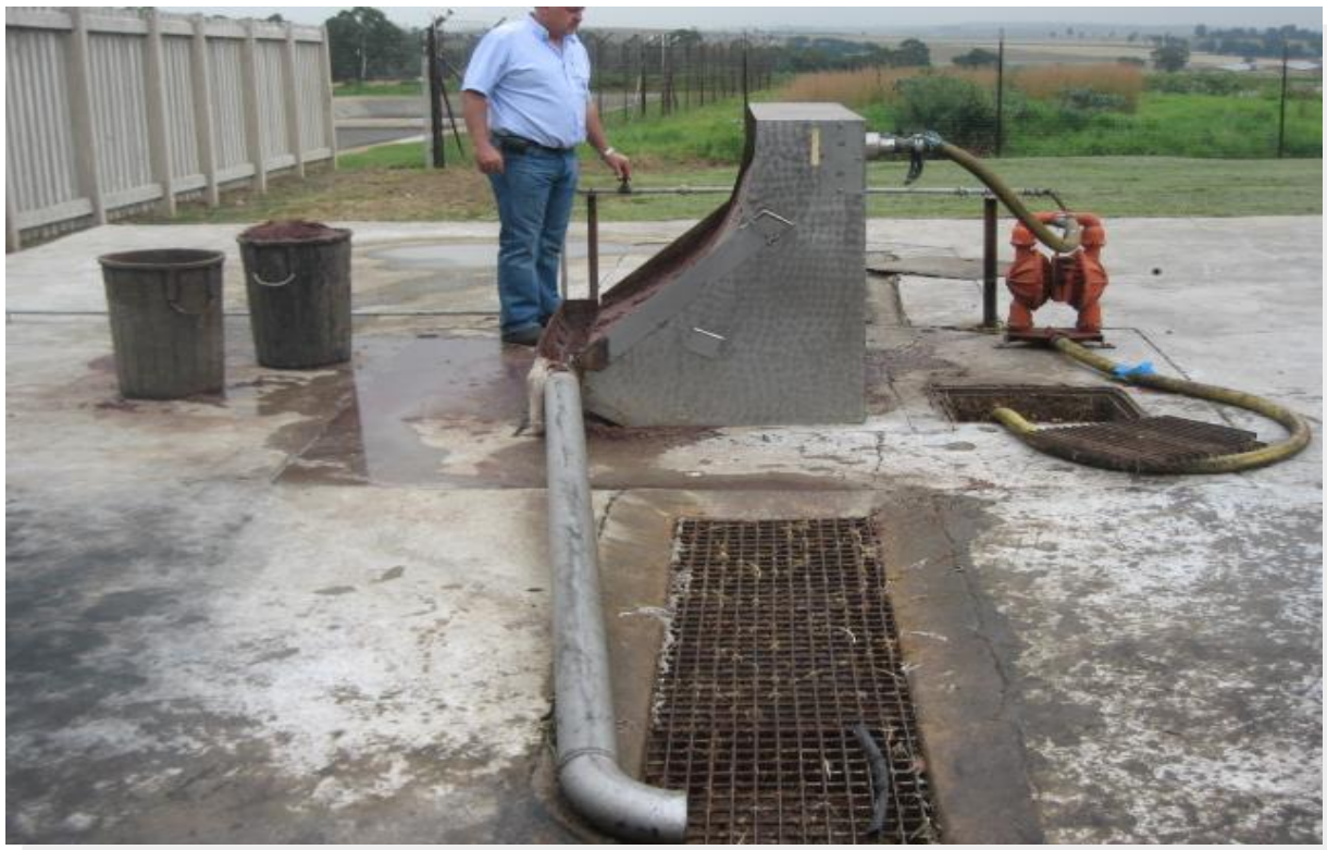
Figure 17: The wastewater collection sump and press. Solids from the press are taken back to the storage bunker
