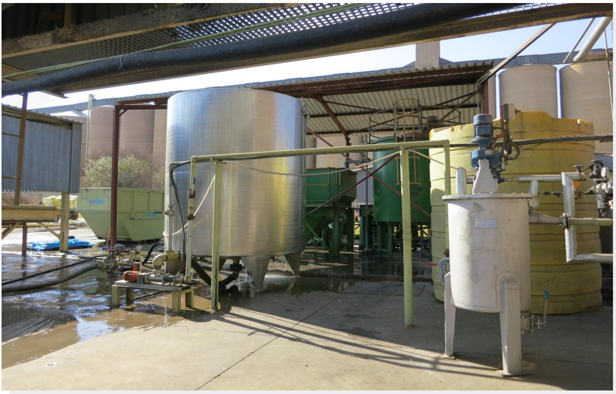
Figure 19: The current blood storage tank
