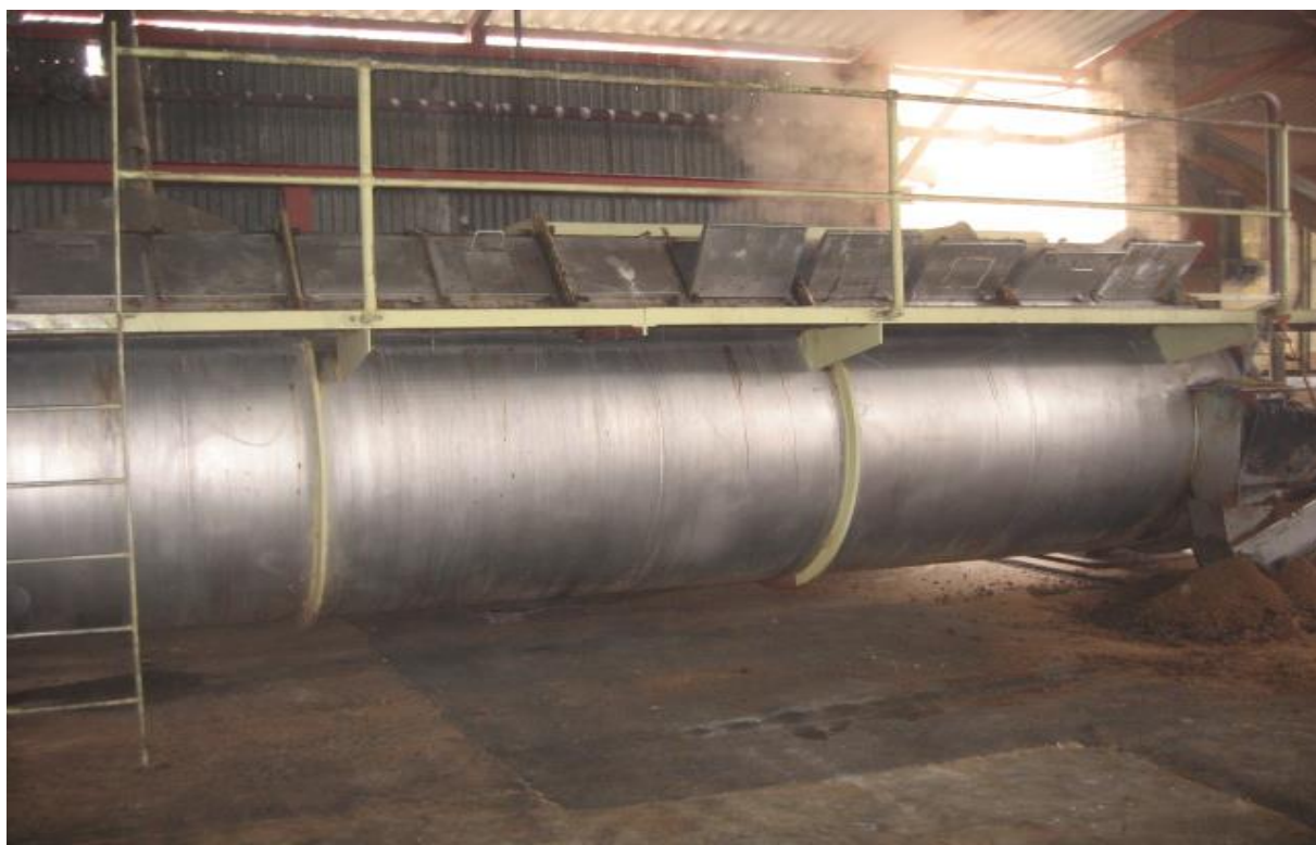
Figure 24: The current dryer where the product is dried to further decrease the moisture content
