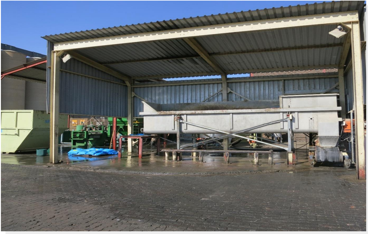
Figure 18: The current hopper into which poultry waste is loaded
