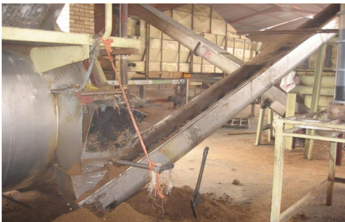
Figure 25: Dried product exiting the drier and passing through the sieve
