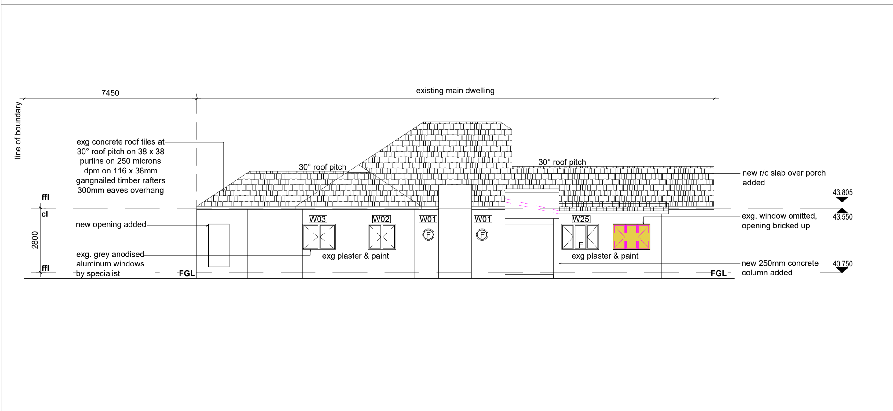
WEST ELEVATION MAIN DWELLING SCALE 1:100
