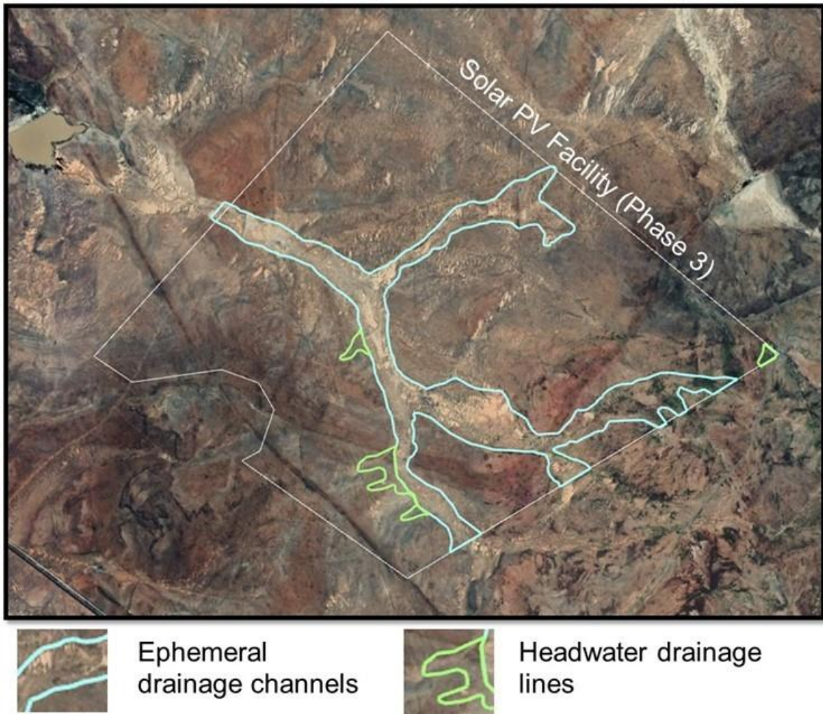
Figure 22: The delineated riparian zone of the Phase 3 PV facility: Green lines - Headwater drainage lines; Blue lines – Ephemeral drainage channels.
