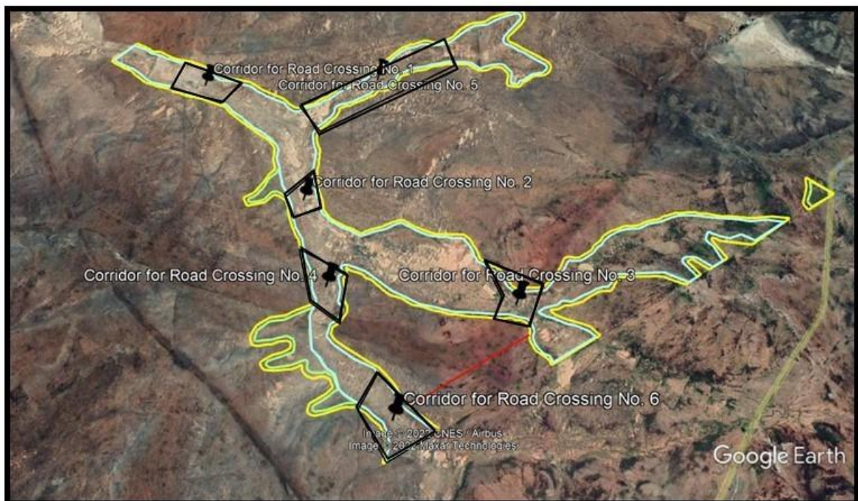
Figure 30: 'Corridors' indicating the permissible area (black polygons) for the alignment of the road crossings (MacGregor, 2022)
