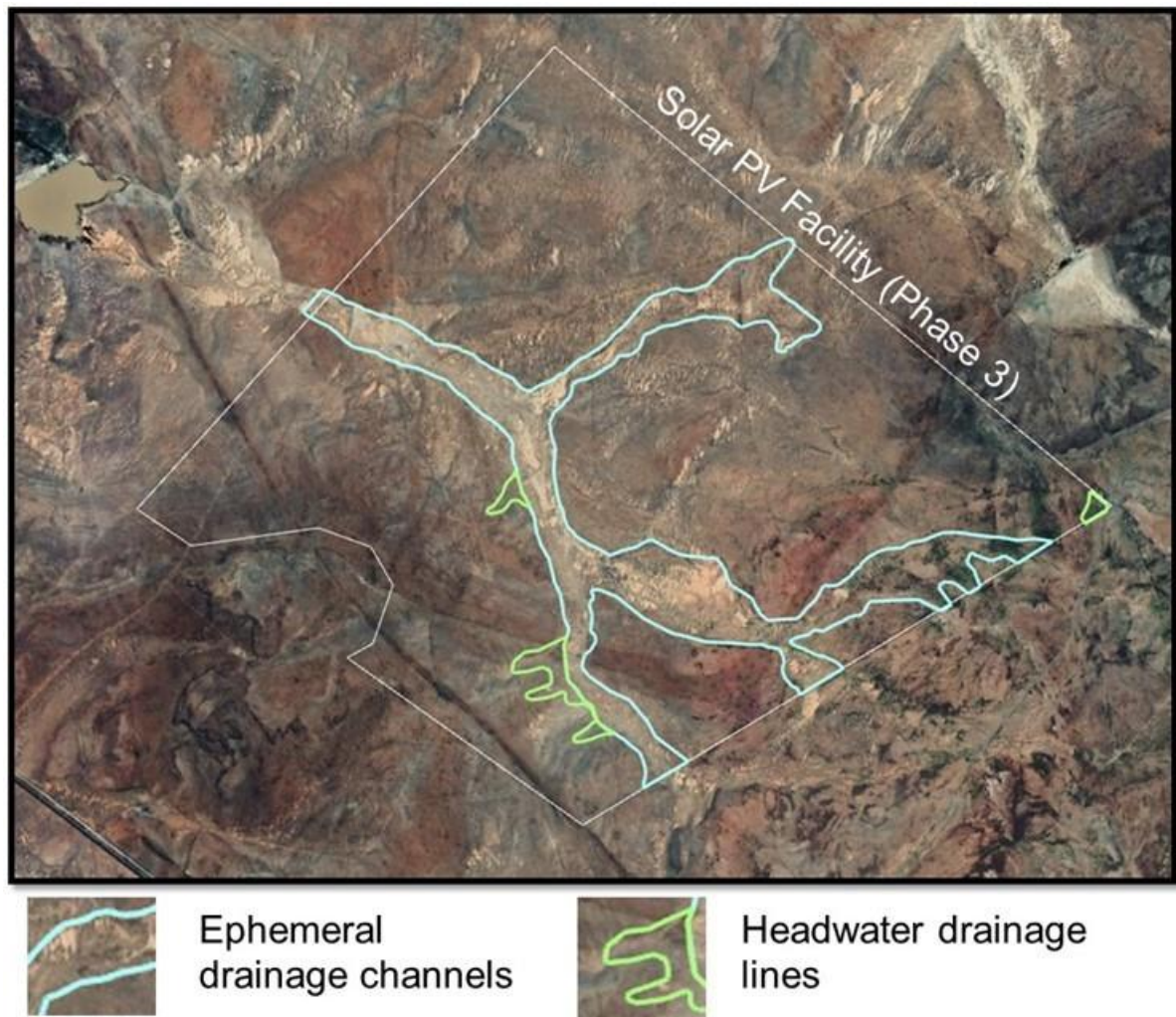
Figure 10: A diagram to identify the different drainage types encountered in the ephemeral drainage system during the aquatic surveys in the project area:
