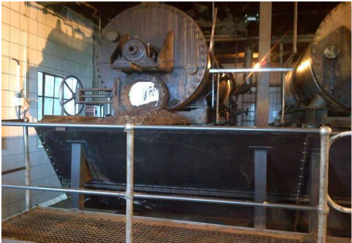
Figure 13: The cooking vessels and offloading area (where the product is removed from the vessels)
