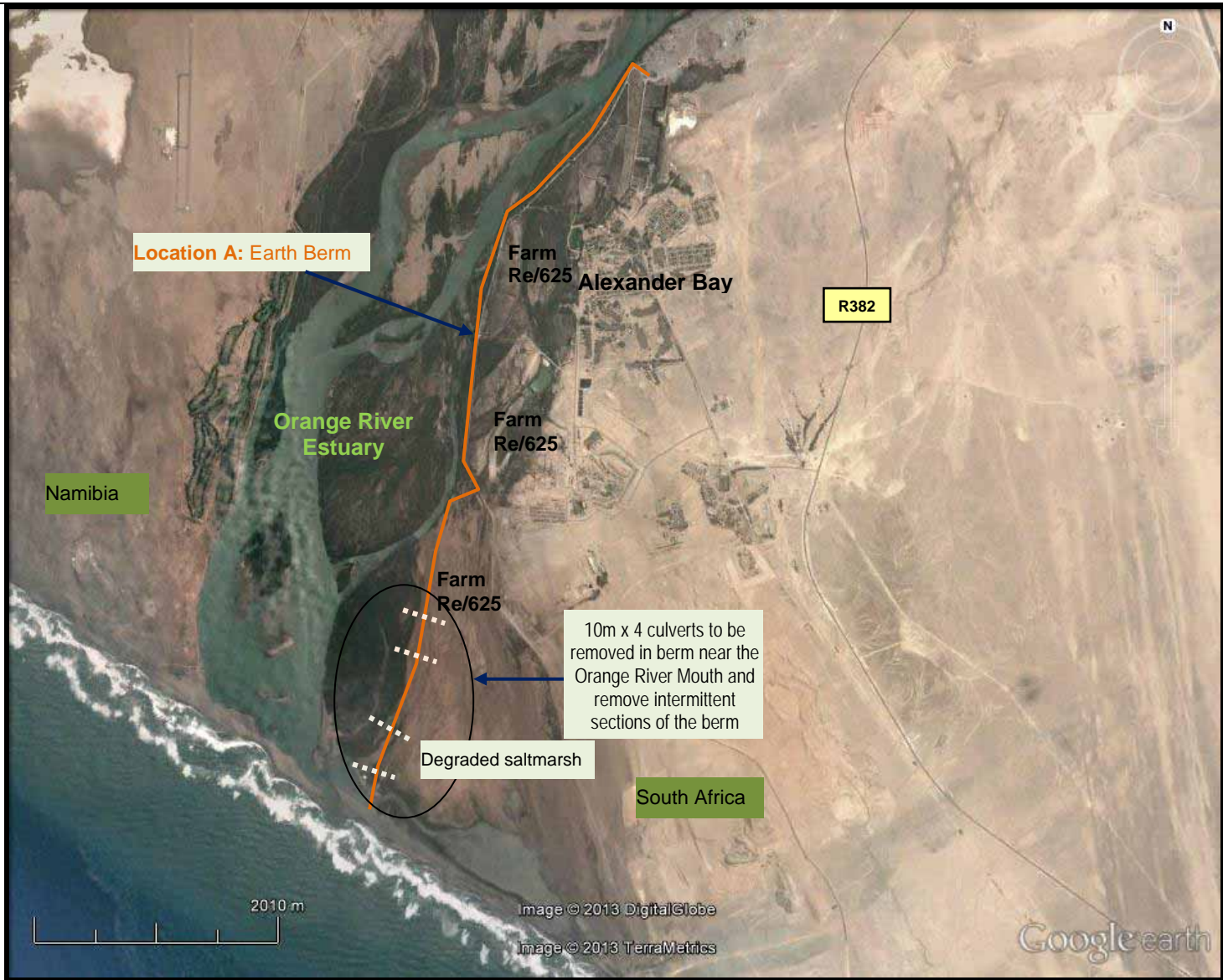
FIGURE 3: PROPOSED ALTERNATIVE DESIGN FOR REMOVAL OF EARTH BERM AT "LOCATION A", ORANGE RIVER ESTUARY, FARM REM /625, ALEXANDER BAY, NORTHERN CAPE.
