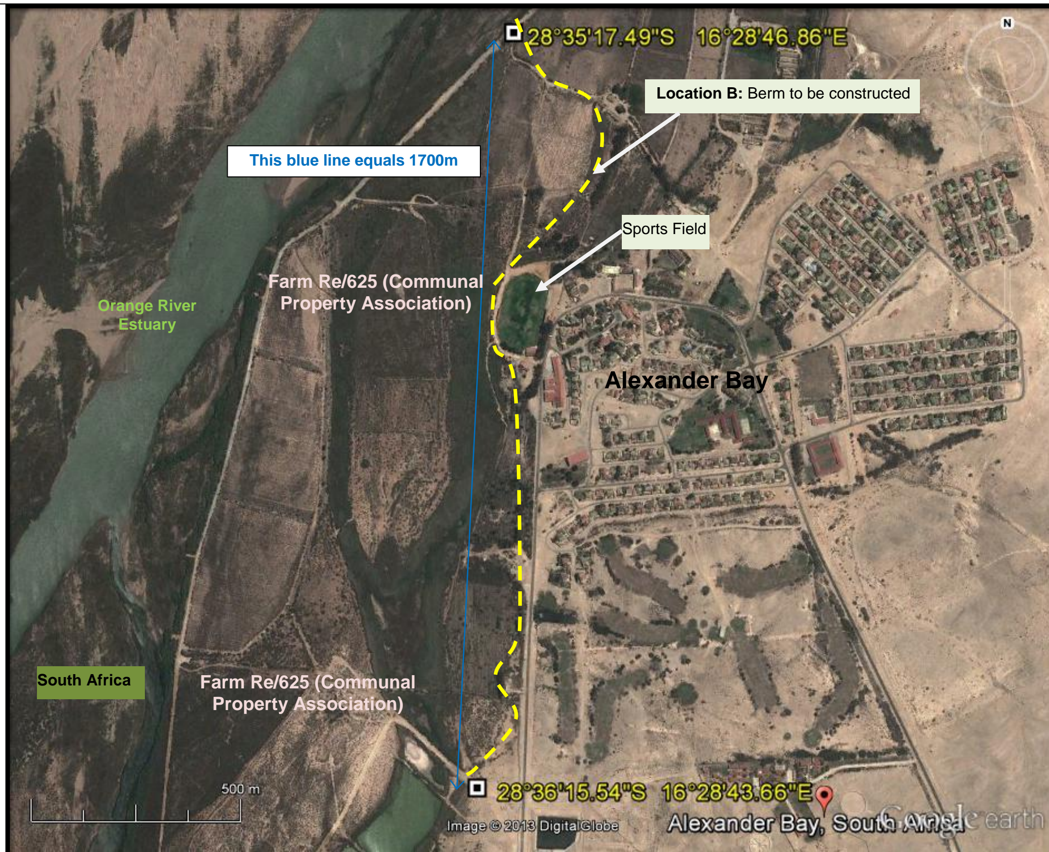
FIGURE 6 GOOGLE EARTH MAP INDICATING THE PROPOSED ROUTE FOR THE CONSTRUCTION OF THE BERM AT "LOCATION B" ON FARM REM/625, ALEXANDER BAY.
