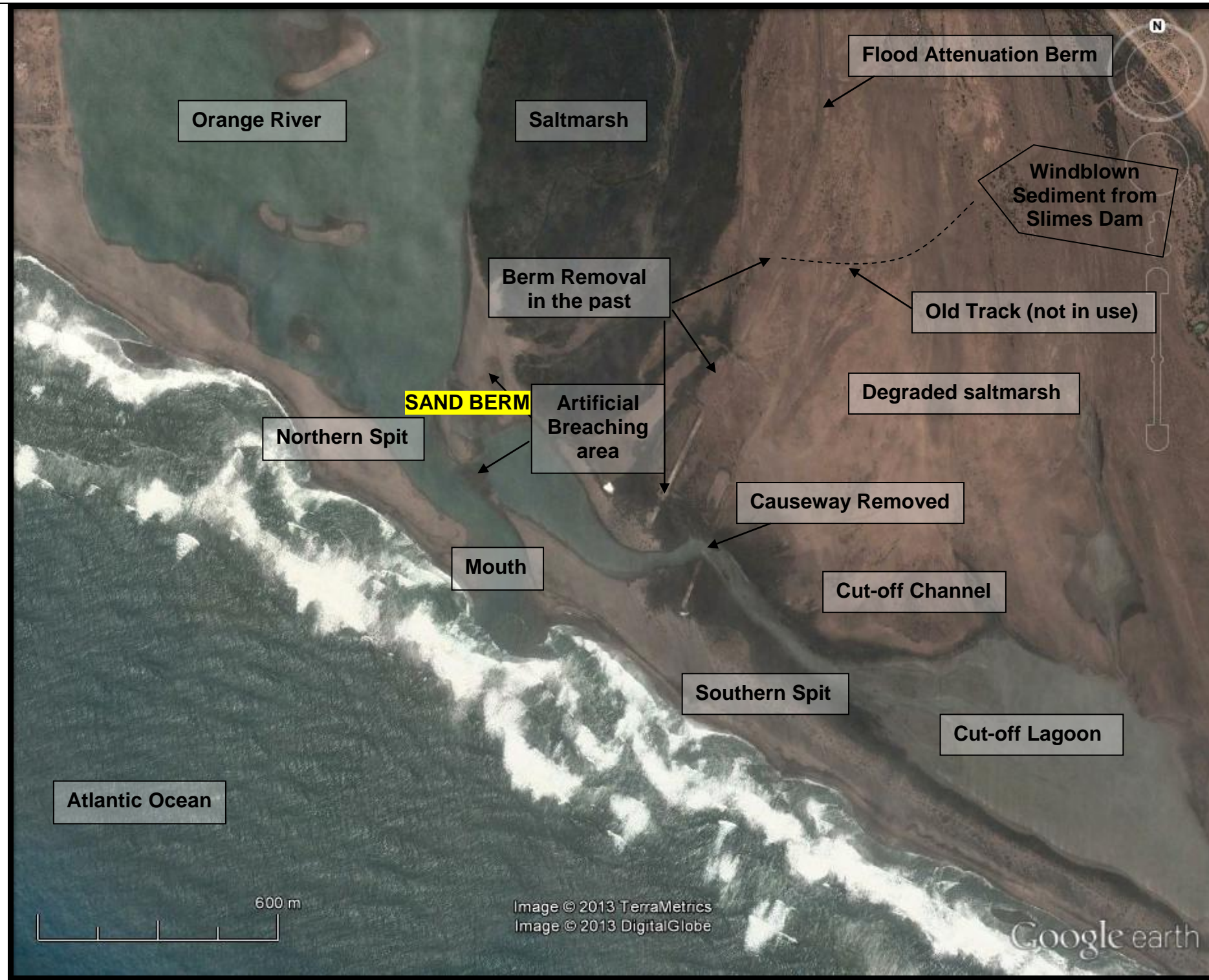
FIGURE 7 GOOGLE EARTH MAP INDICATING THE PROPOSED ARTIFICIALLY BREACHING OF THE SAND BERM ACROSS THE FLOOD CHANNEL TO THE SOUTH OF THE ORANGE RIVER MOUTH (LOCATION C).
