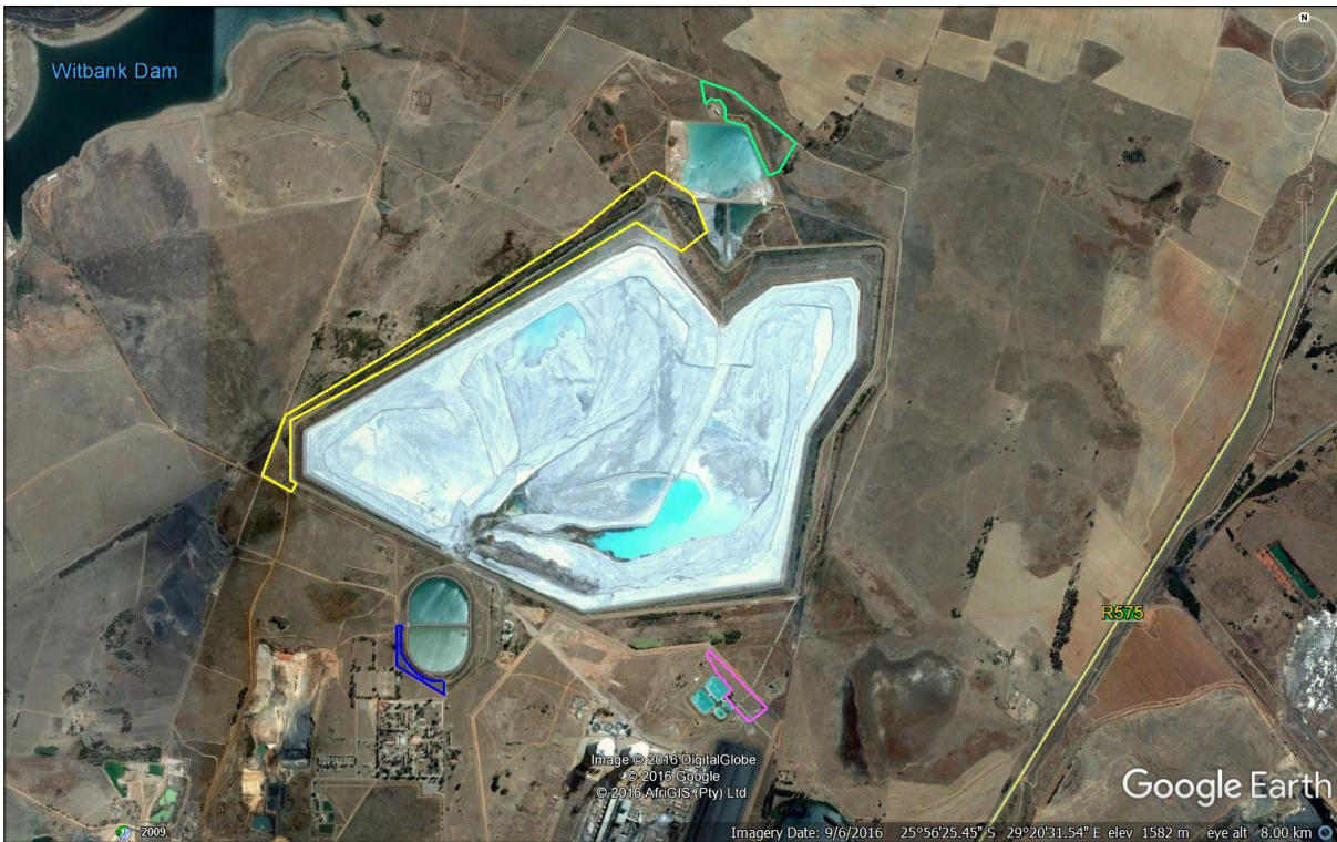
Figure 3: Google Earth image showing the proposed servitude footprint areas for the seepage interception drains (yellow, green, blue and pink polygons) (Map provided by Nema Consulting, 2017).
