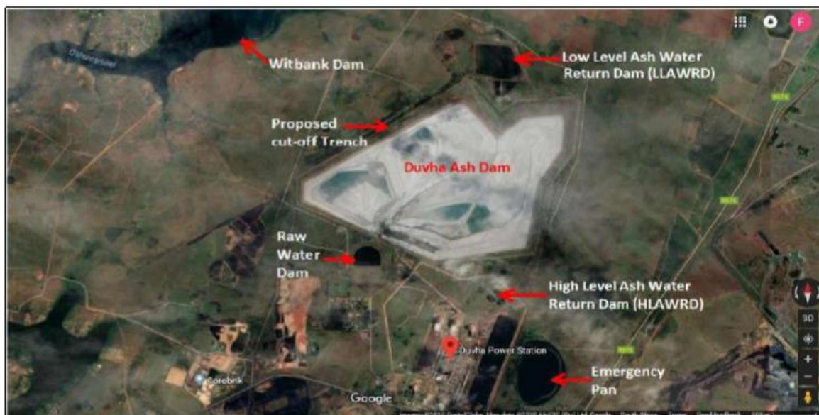
Figure 1: Site layout of the Duvha Power Station, indicating the location of the affected return water dams in relation to the Ash Dam (Map provided by Eskom, 2019)
