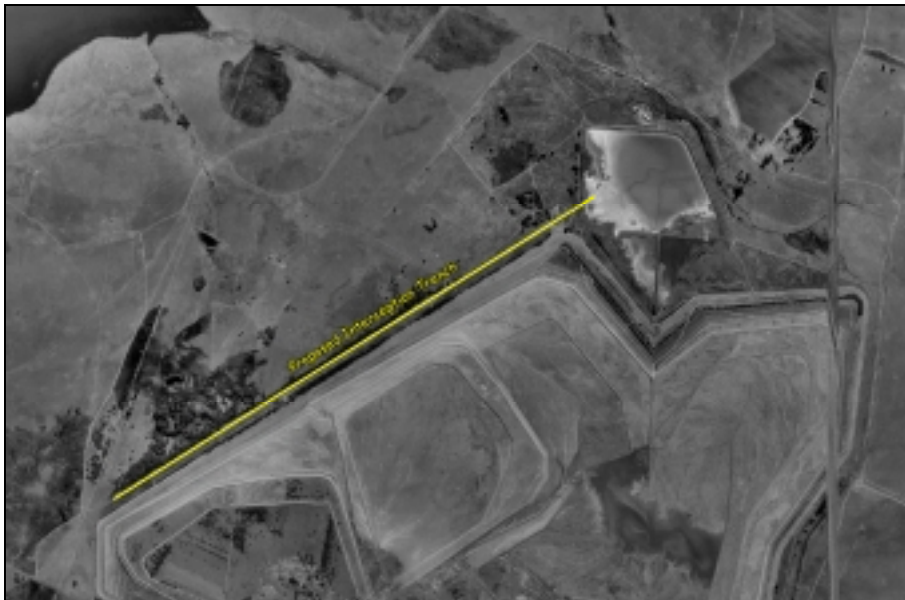
Figure 42. Location of the proposed seepage interception trench north of the Ash Dam.
