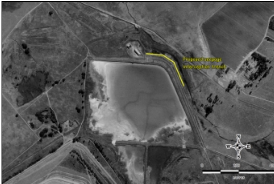
Figure 45. Position of possible seepage interception trench at the Low Level Ash Water Return Dam.
