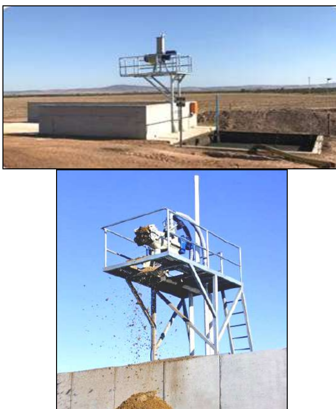
Photo 7.5: An example of a screw-press separator (obtained from Big Dutchman and www.sajWare.com ).
