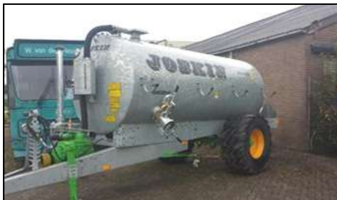
Photo 7.9: An example of the tractor and tanker to be used for the spreading of manure
