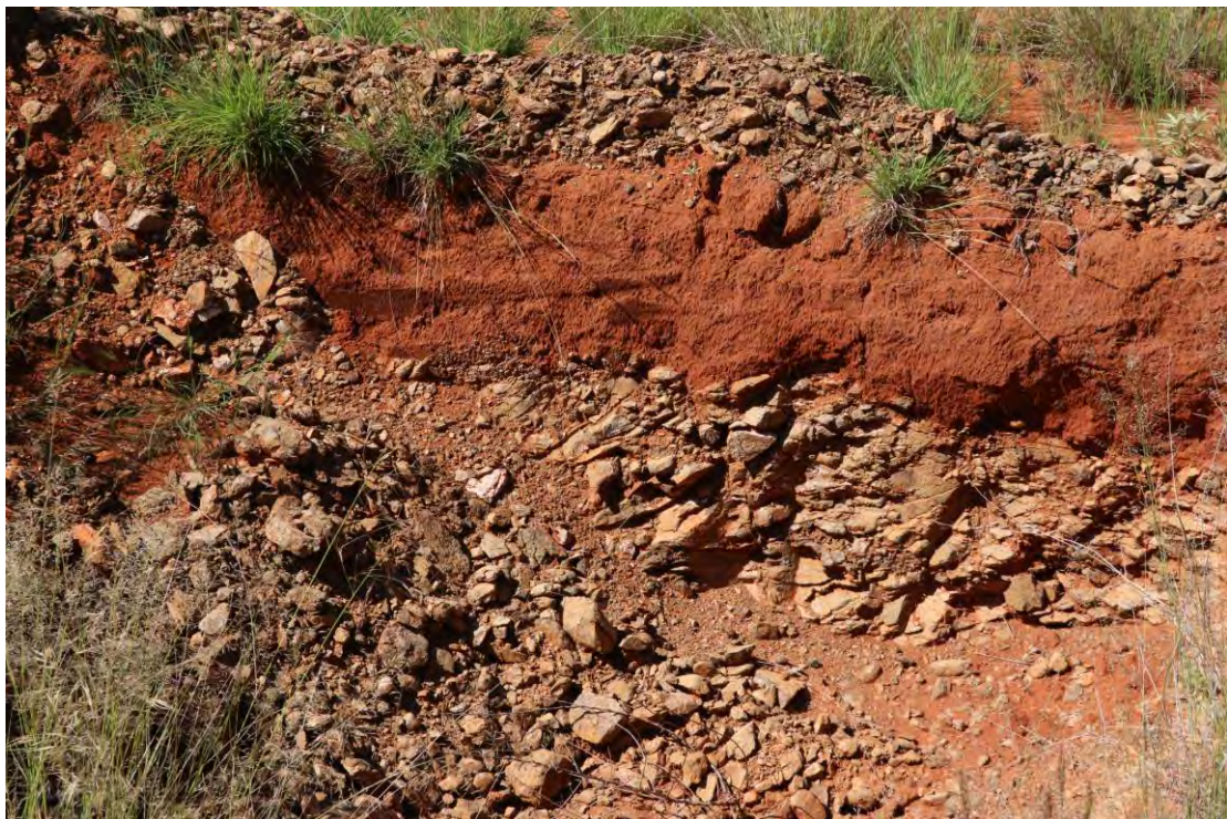
Figure 6: View of the soil profile at the site indicates a shallow topsoil layer, dominated by sandy-loam soils overlying weathered dolerite.
