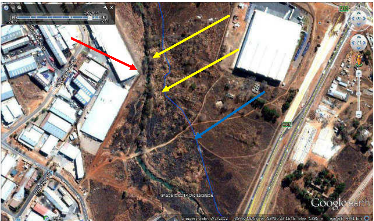
Figure 24 Encroachment of infrastructure on the Rietspruit (red arrow) as well as historical rubble dumping (yellow arrows) with sewer line transect indicated in blue
