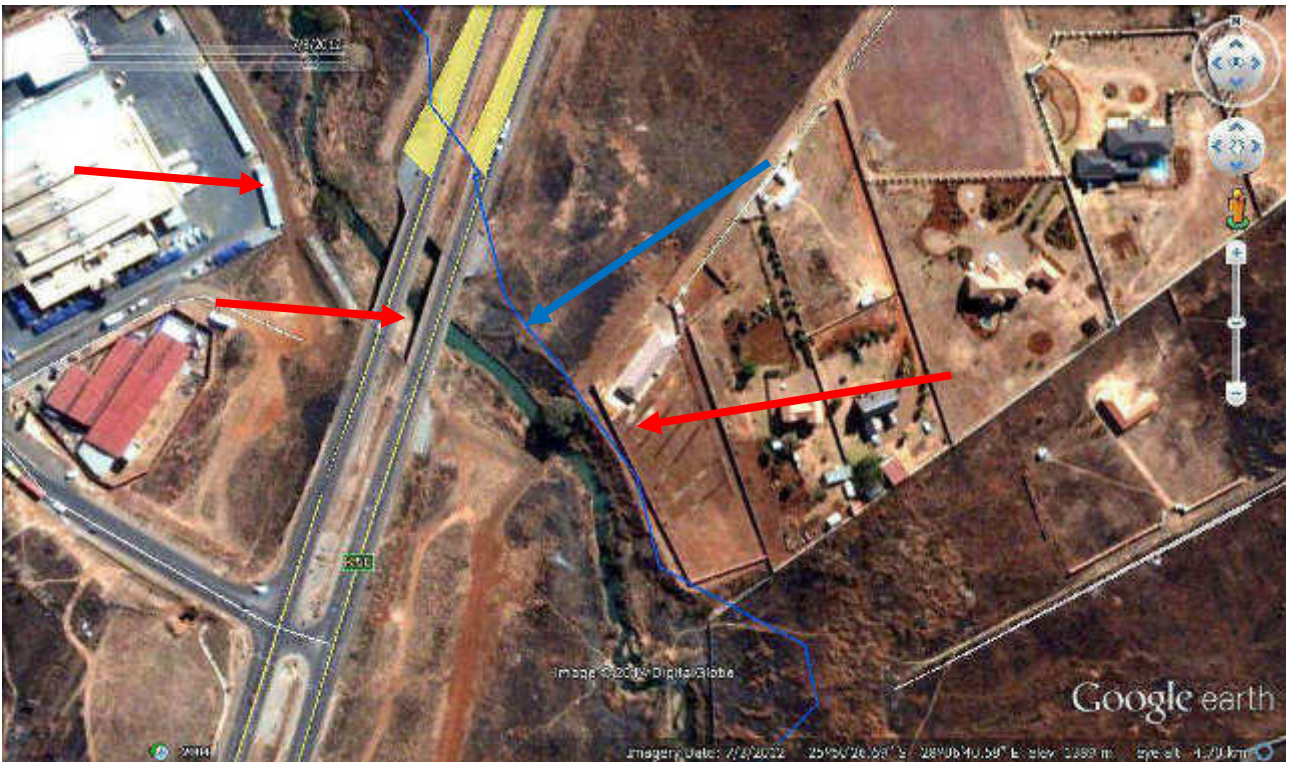
Figure 23 Encroachment of infrastructure and cut and fill activities on the Rietspruit (red arrows) (sewer line transect indicated in blue)
