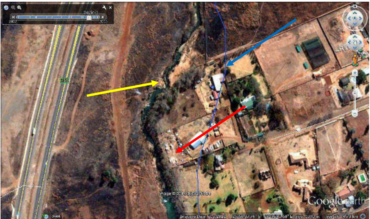
Figure 22 Sedimentation (yellow arrow) near the end of Deltoidia street as well as encroachment of human activities on the Rietspruit (red arrow) (sewer line transect indicated in blue)
