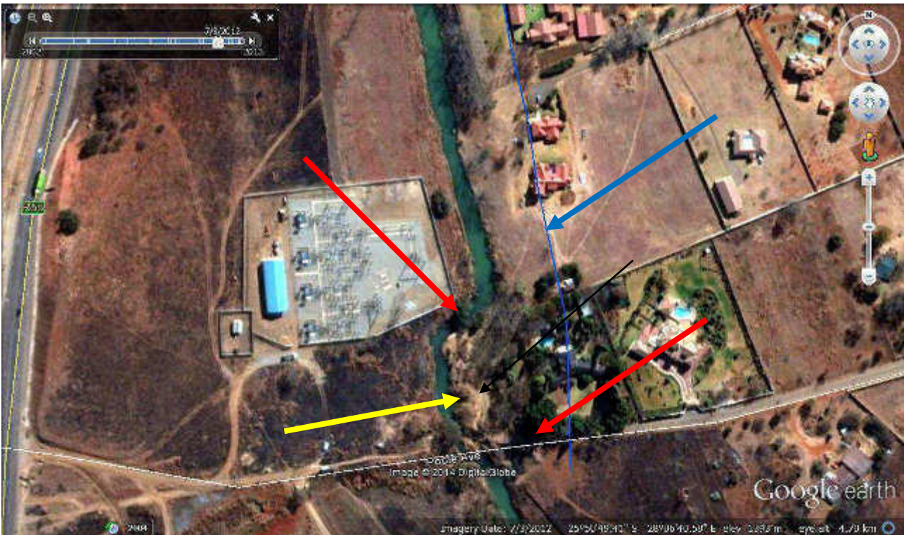
Figure 21 Sedimentation (yellow arrow) at the end of Poole avenue as well as encroachment of infrastructure on the Rietspruit (red arrows) (sewer line transect indicated in blue)
