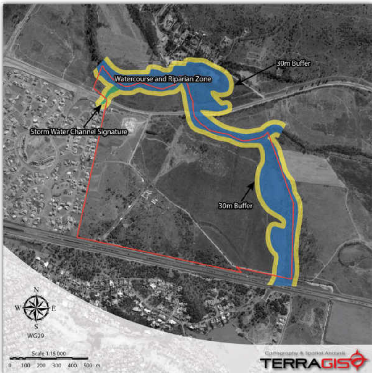
Figure 34 Wetland area on the site
