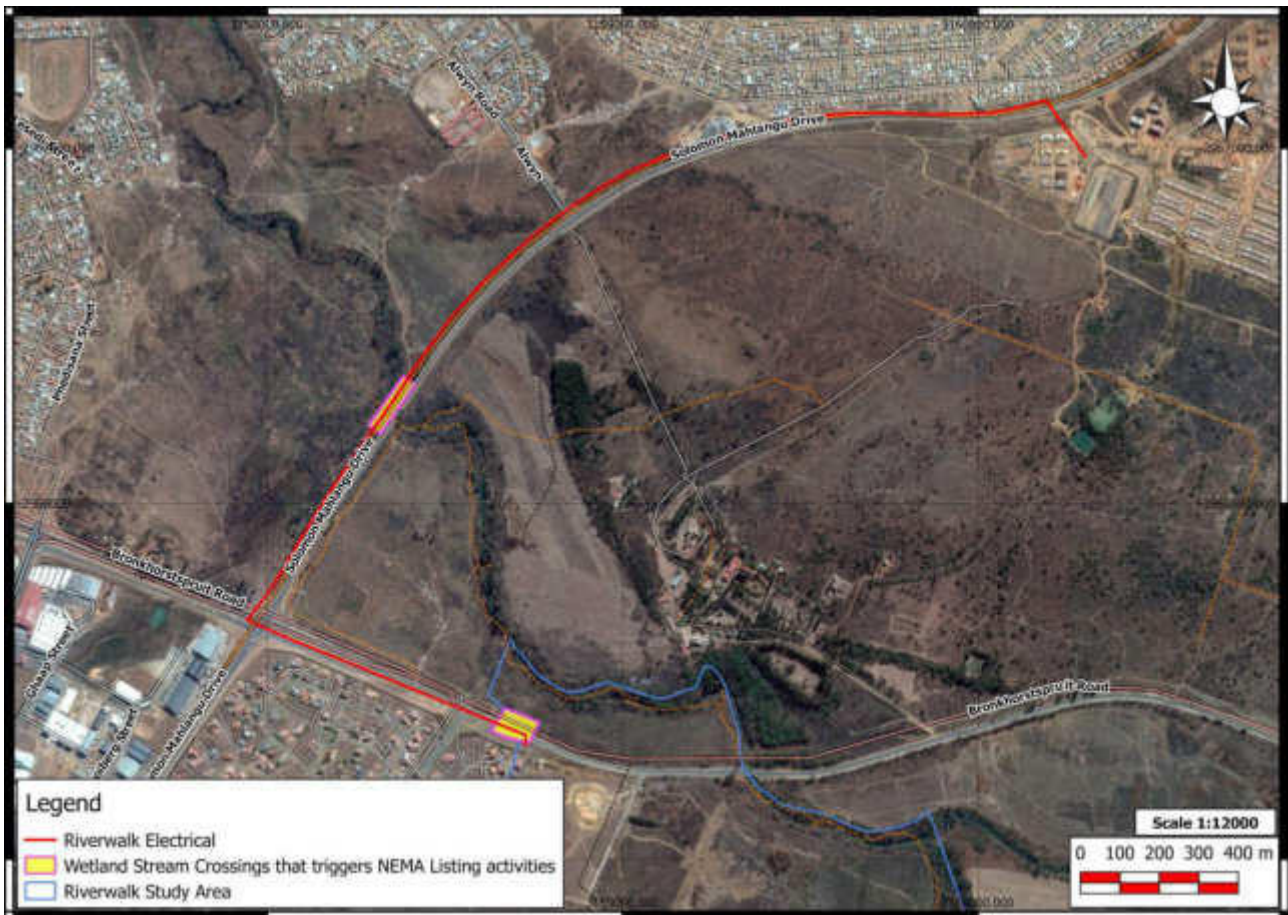
Figure 40 Electrical infrastructure for the development running in the road reserve and crossing a wetland / storm water structure
