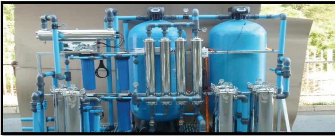
Fig 5: Proposed water purification system
