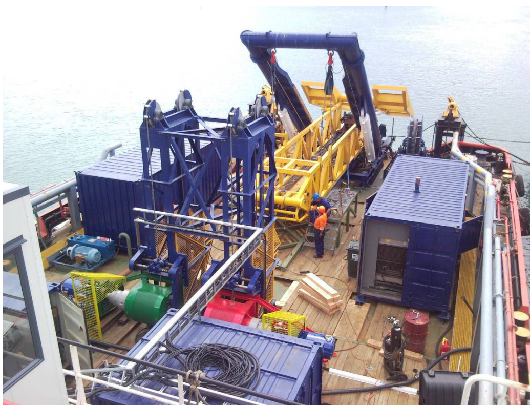
Figure 3.2: AuruMar’s Sonic VibroCorer on a vessel.
