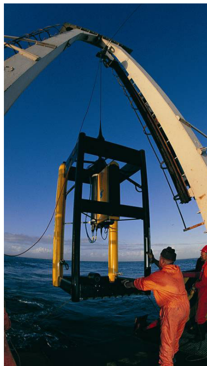
Figure 3.3: Focus Towfish could be used to collect both side scan sonar and Chirp seismic data.
