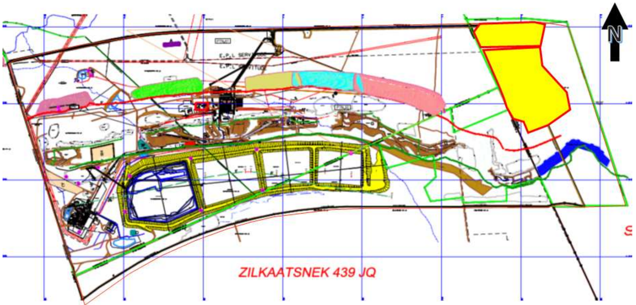
Figure 7: Locality of the PV Project Area in relation to the Existing Mining and Surface Infrastructure.
