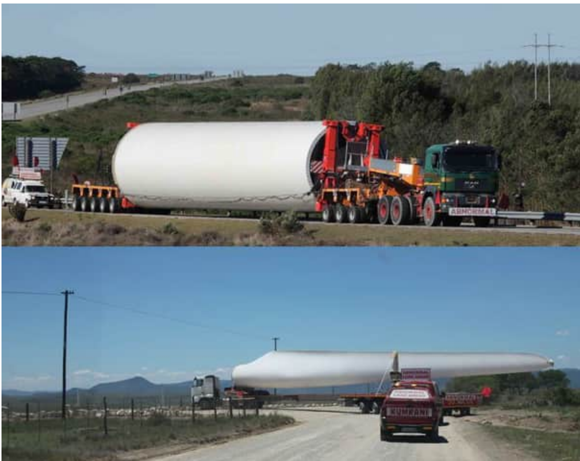
Figure 2-18: Tower section in low load configuration shown in top figure and blade shown in bottom figure
