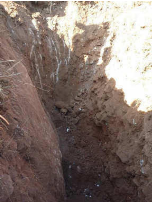
Figure 15 Deeper soil profile with dolomite rock to the left and chert rocks and pebbles in the matrix
