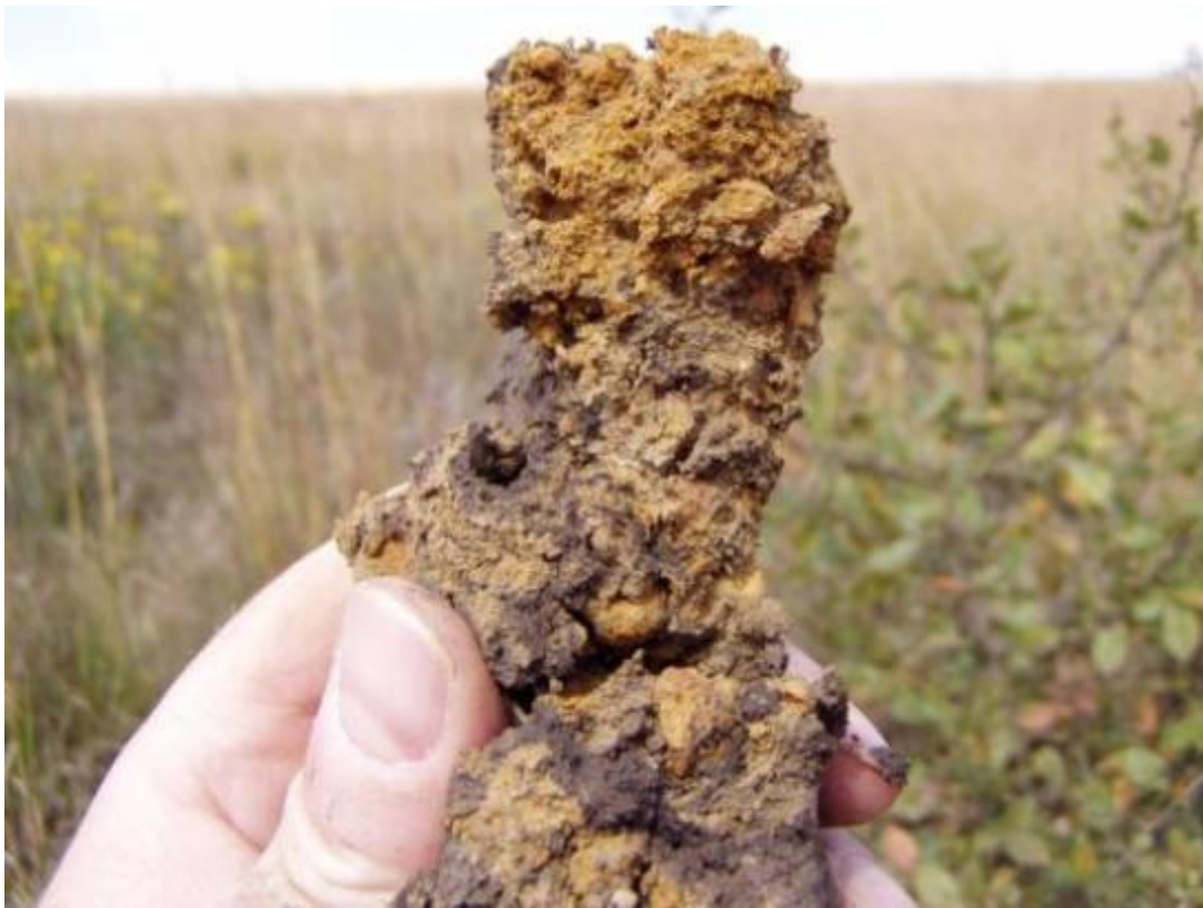
FIGURE 6:24 – EXAMPLE OF SOILS FROM A SOFT PLINTHIC B HORIZON ENCOUNTERED WITHIN THE WETLAND
