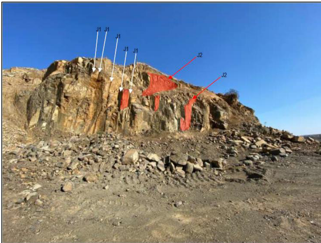
Figure 47: Image showing the joint sets exposed at the southern outcrop at Wansley Quarry (image obtained from the Mining Plan).
