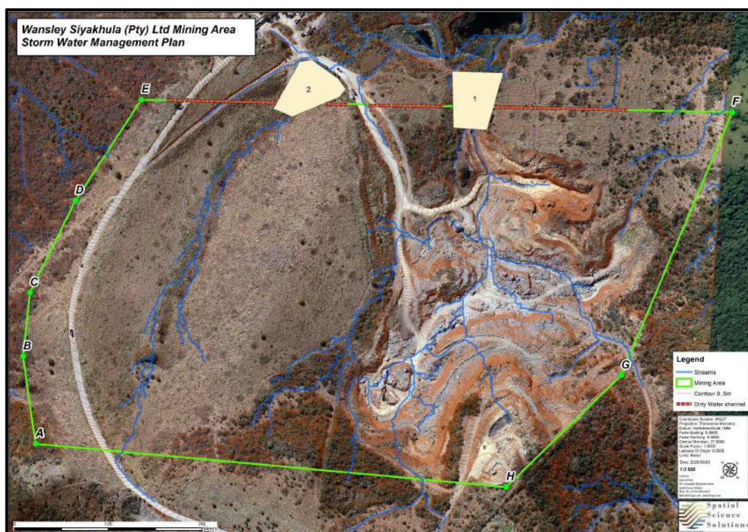
Figure 10: Image showing the drainage lines within the mining footprint (blue lines) as well as the proposed position of the stormwater dams (light yellow polygons) (image obtained from the SWMP).
