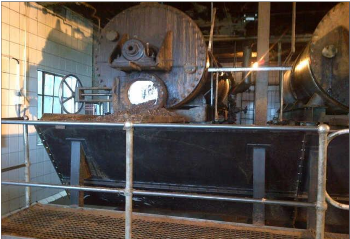
Figure 12: The cooking vessels and offloading area (where the product is removed from the vessels)
