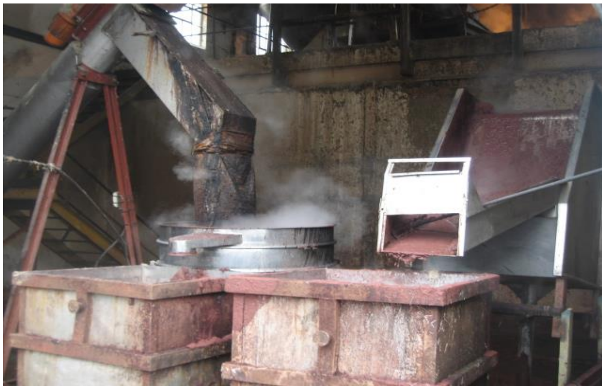
Figure 20: The current blood coagulator where the blood is coagulated before it is added to the poultry waste in the bunker
