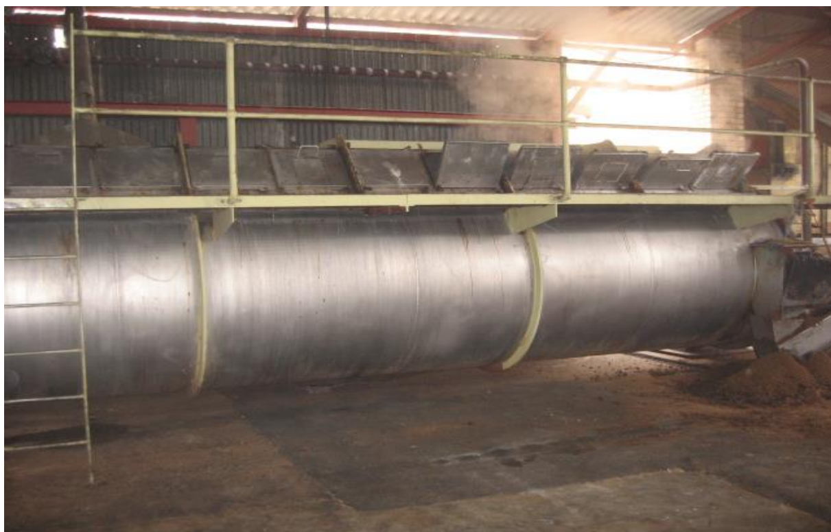
Figure 24: The current dryer where the product is dried to further decrease its moisture content
