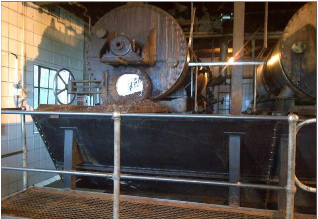
Figure 12: The cooking vessels and offloading area (where the product is removed from the vessels)
