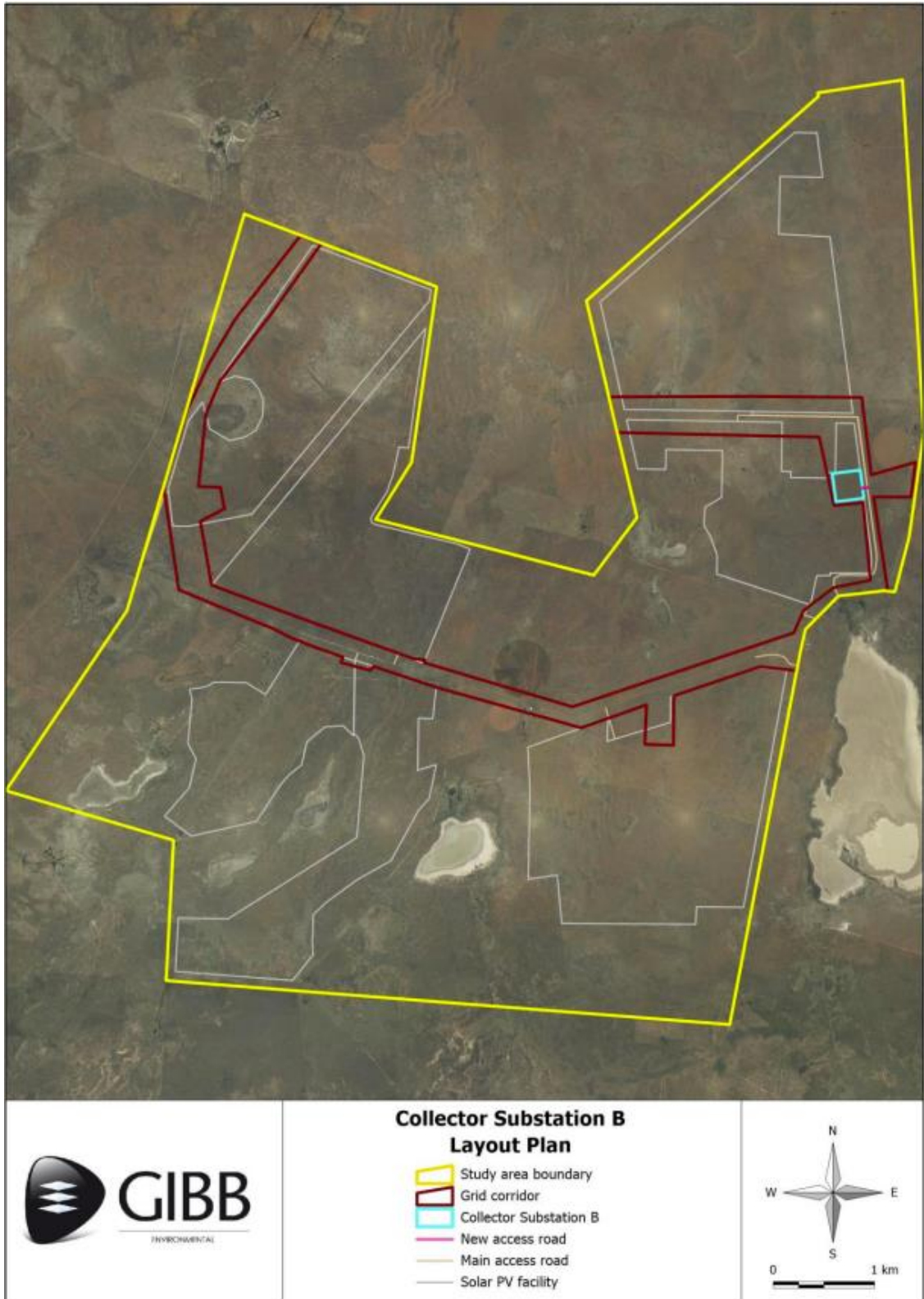
Figure 2-1: Collector Substation B Layout Plan
