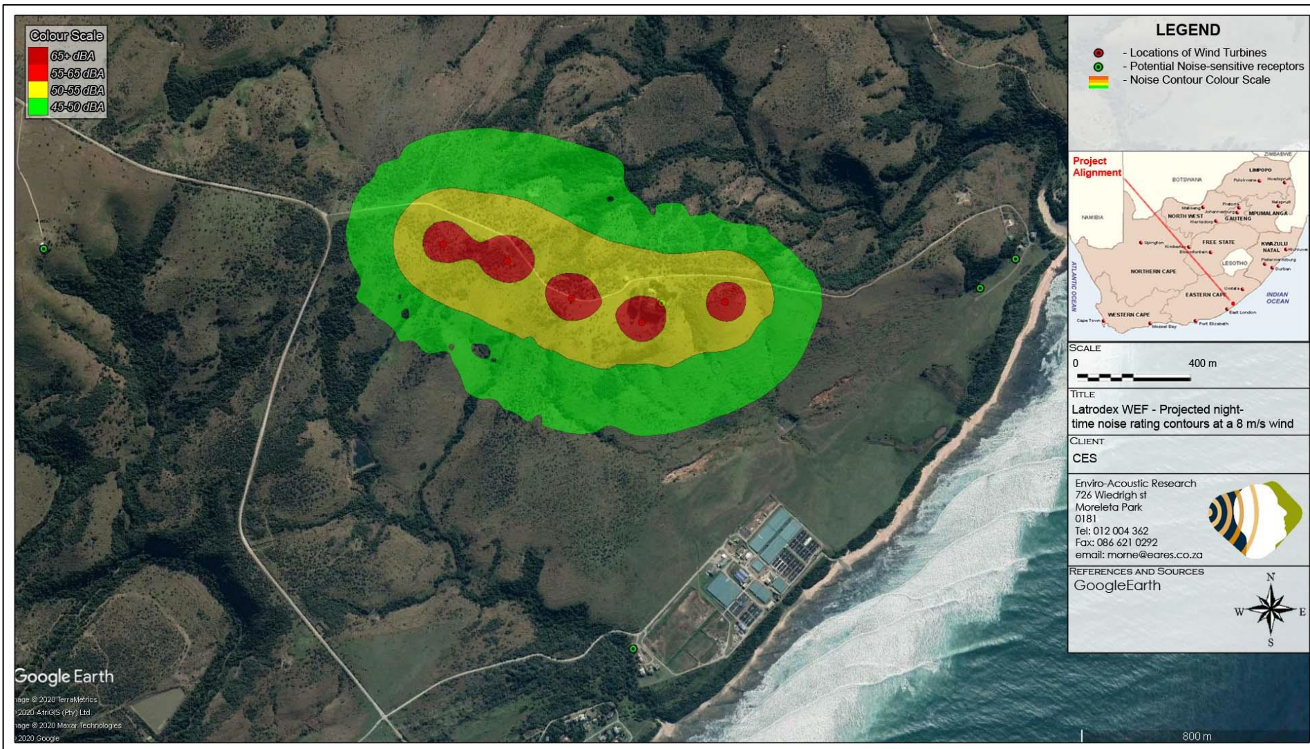
Figure 9-3: Projected conceptual noise rating levels of the Latrodex WEF during operation using the Vestas V90 WTG
