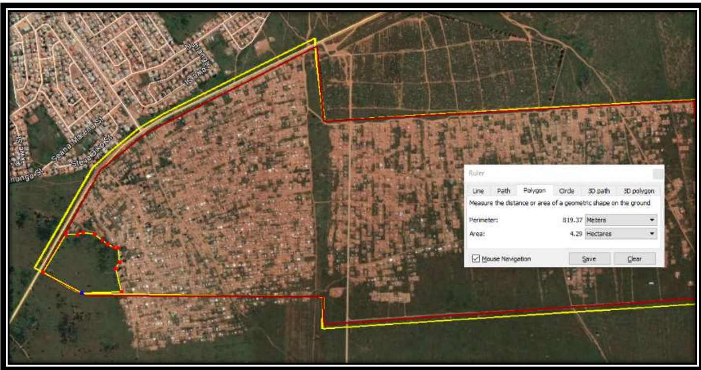
Figure 5: Eradication of indigenous vegetation at the western portion of the development. Total area of 4,29 hectares will be eradicated on this portion.
