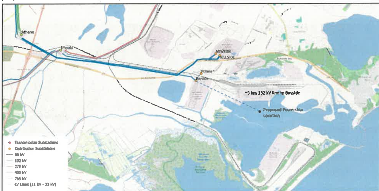
Figure 3-5: 132kV connection at Bayside Substation in relation to the location of the Powership
