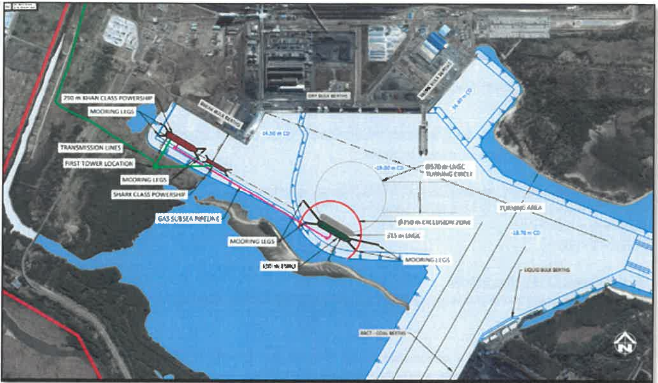
Figure 3-3: Alternative 1: Powership and FSRU position within the port – closer to transmission tower
