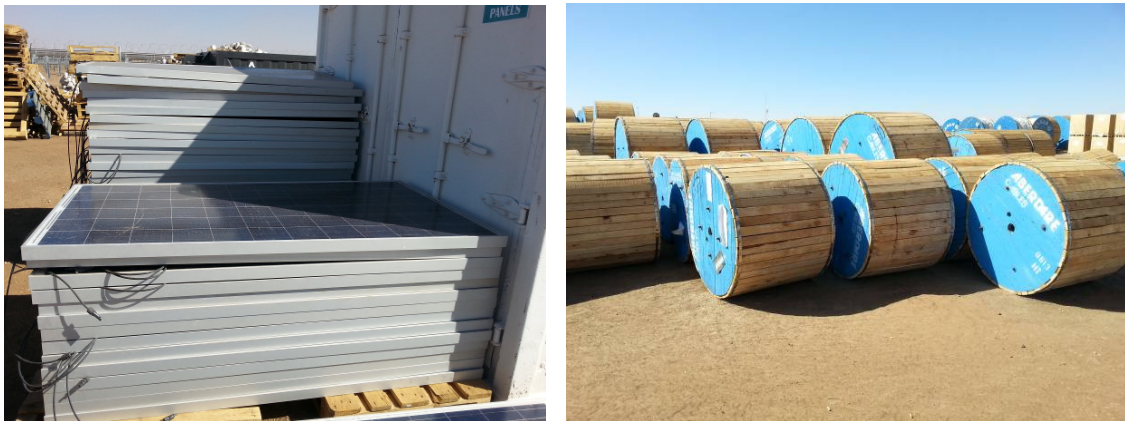
Figure 8 (a & b): Figure A shows an example of the storage of a PV Solar Panels once taken out of the box packaging. Figure B shows an example of the storage of cables
