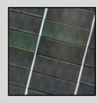
Copper, Indium, Gallium, Selenide (CIGS) - CIGS is a compound semiconductor that can be deposited onto many different materials. CIGS has only recently become available for small commercial applications, and is considered a developing PV technology (First Solar, 2011).
