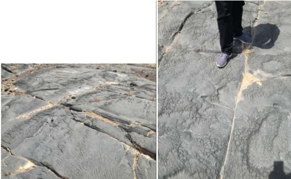
Photo 1 (a and b): Outcrops of thickly bedded black dolomite with vertical jointing which hopefully only occurs in the upper layer related to stress release during exfoliation
