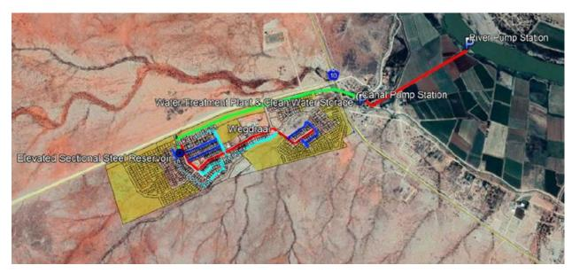
**Figure 23**. Current water supply system associated with the existing Wegdraai Settlement. Source: Engineer's Service Report (Appendix 4B).
