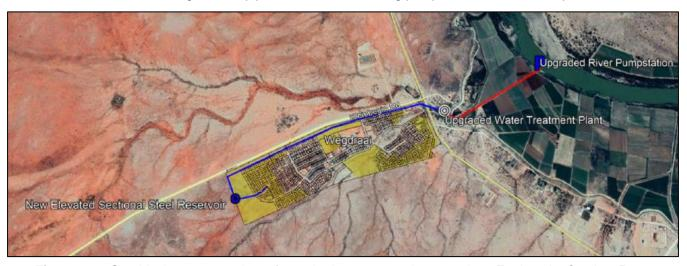
**Figure 24**. Graphical representation of required water supply upgrades. Engineer's Service Report (Appendix 4B).
