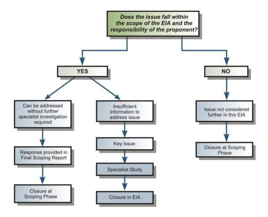
Figure 6.1 Decision-making framework for identification of key issues for the EIA
