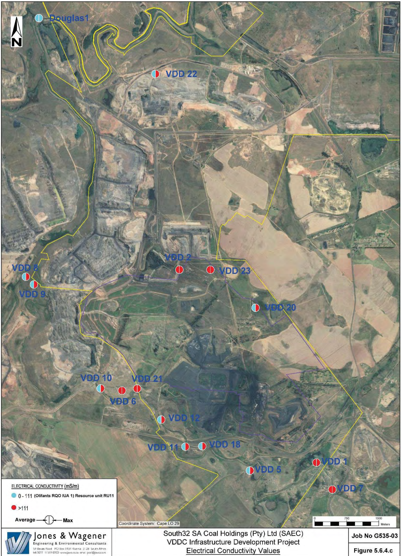
Figure 10-12: Electrical conductivity (EC) levels measured at surface water monitoring locations (J&W, 2018c)
