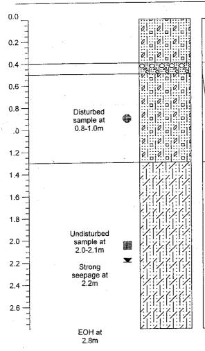
SILTY SAND AND SCATTERED GRAVEL: Moist, dark greyish brown. LOOSE, intact silty sand, with scattered gravels and roots. Hillwash
