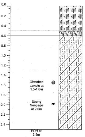
SILTY SAND AND SCATTERED GRAVEL: Moist, dark greyish brown, LOOSE, intact silty sand, with scattered gravels and roots. Hillwash
