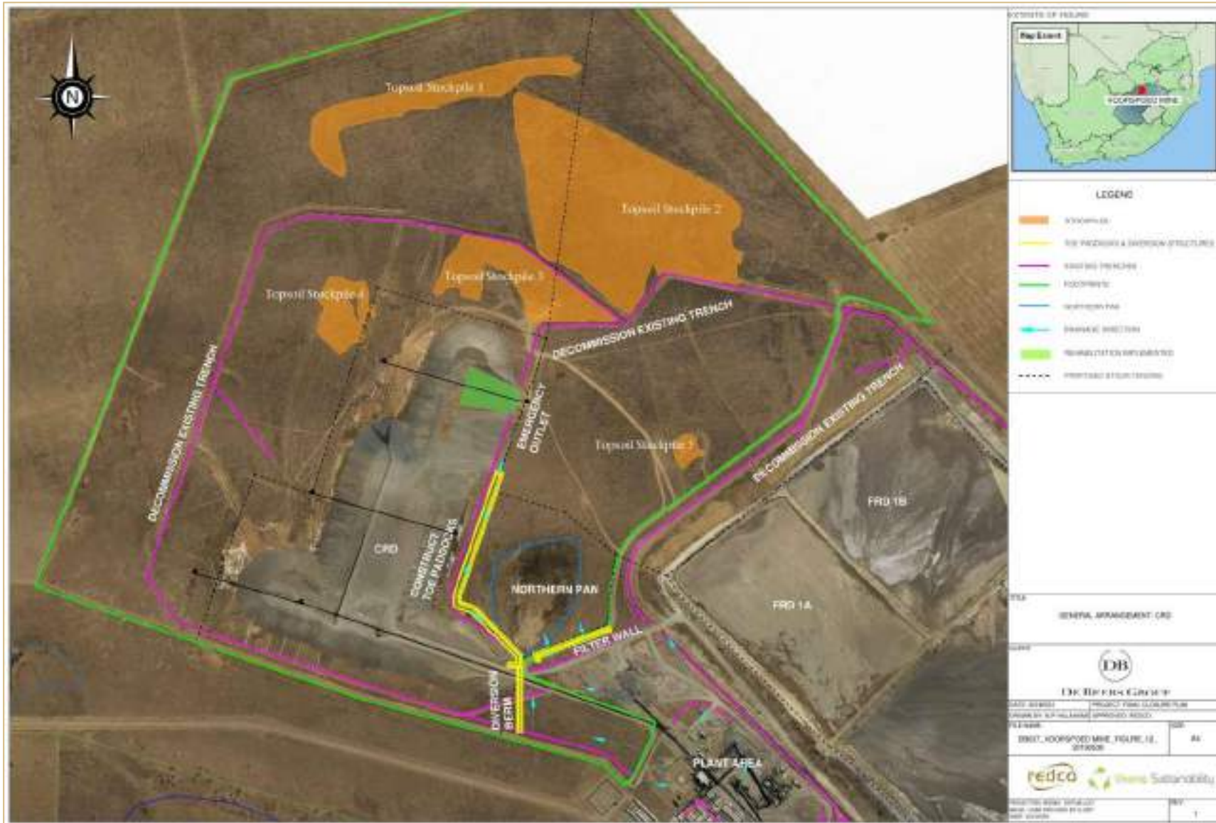
Figure 10: CRD: General Arrangement
