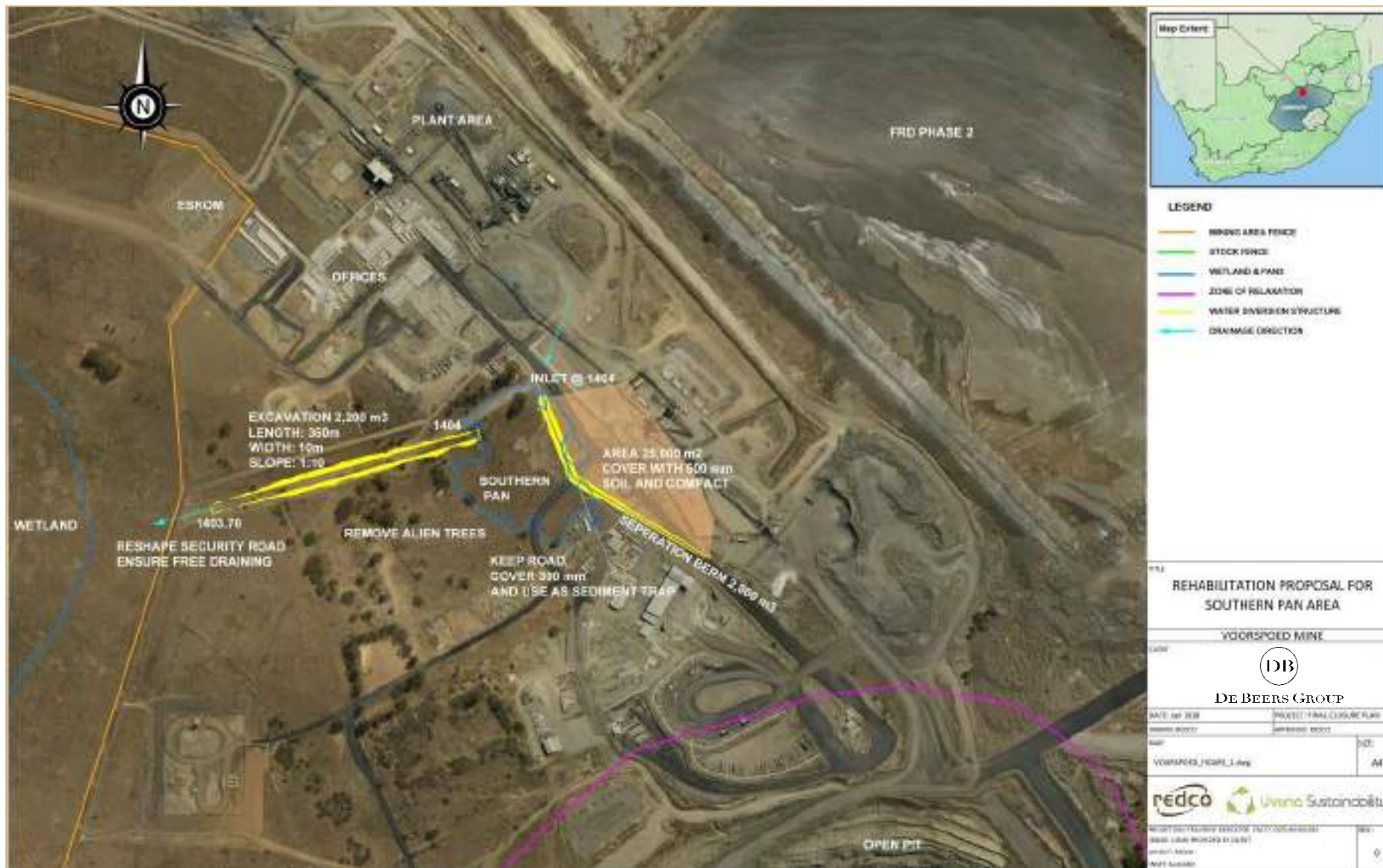
Figure 6: Rehabilitation proposals for the Southern Pan area
