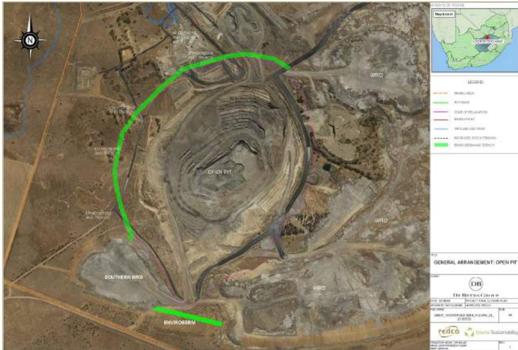
Figure 24: Open Pit – General Arrangement
