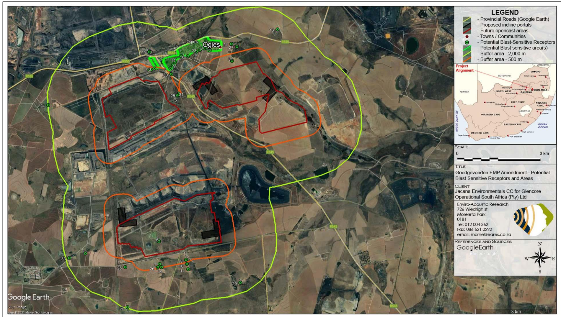
Figure 3-1: Aerial image indicating potential BSR within 2,000 m of potential blasting area (complete potential mining opencast area)
