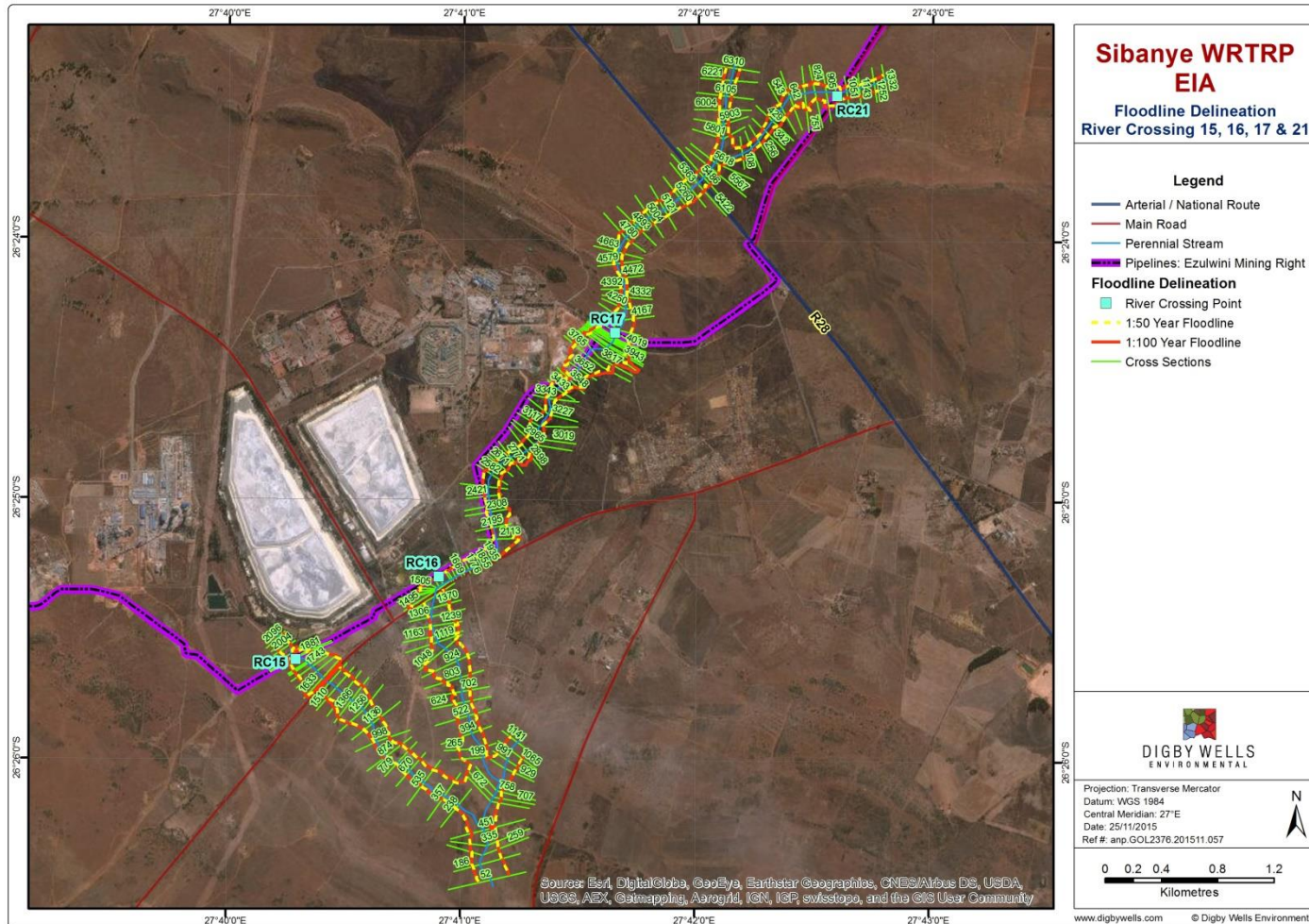
Figure 8-8 1:50 and 1:100 Delineated Floodline for RC15, RC16 and RC17
