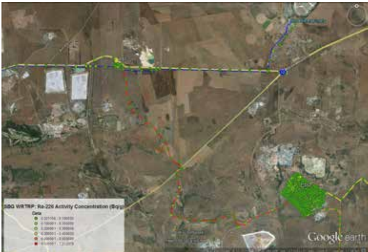
Figure 9-1: Example of gamma spectrometric results reported for the proposed WBT and CPP footprint areas and the associated pipeline routes (NECSA, 2015).
