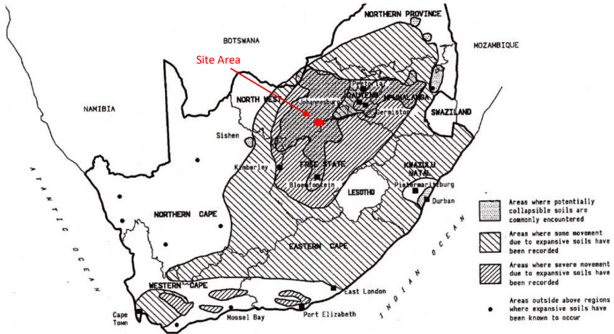
Figure 5-3 Map of potentially unstable soils in South Africa (Taken from NHBRC HBM, 2015)
