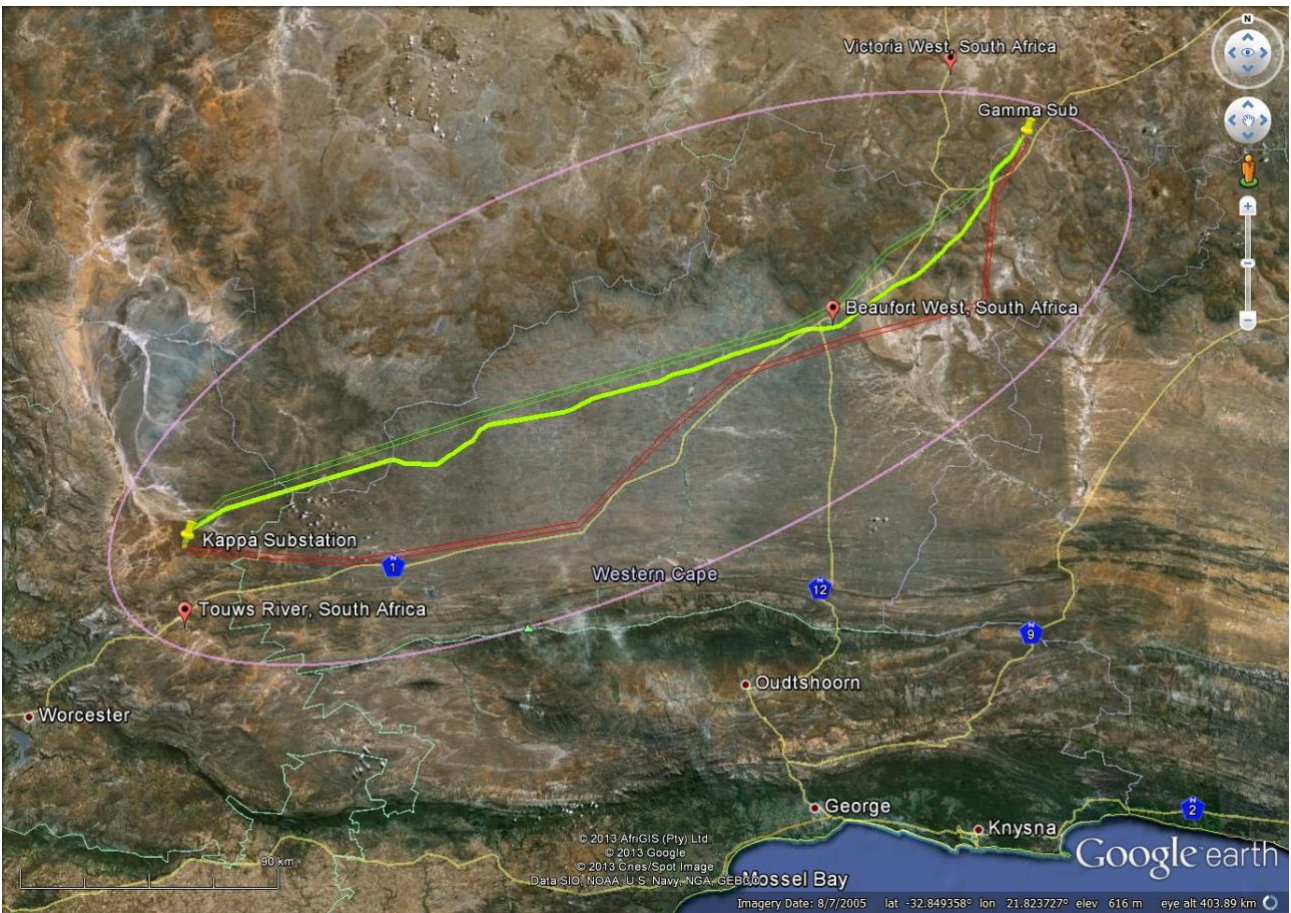
Figure 7: A map indicating alternative 2 (solid green line) which has emerged as the preferred alternative from a bird impact assessment perspective.
