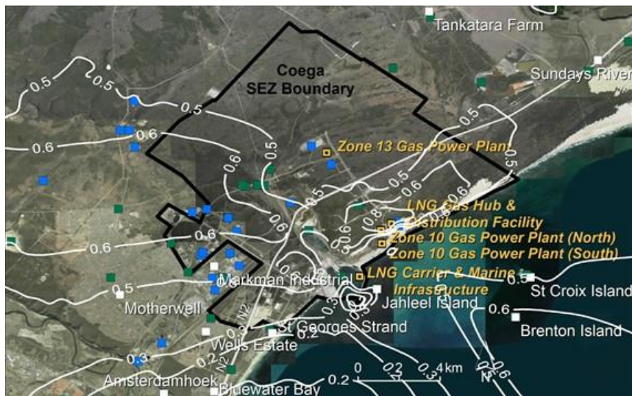
Figure 18: Predicted annual average NO 2 concentrations in µg/m 3 for Scenario 1 the Land-based LNG Terminal and Infrastructure Project (top left), Scenario 2 the Land-based LNG Terminal and Infrastructure Project with baseline (top right), Scenario 3 the 3 000 MW Coega G2P Project (bottom left) and Scenario 4 the 3 000 MW Coega G2P Project and baseline (bottom right)
