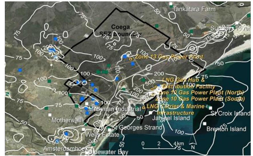
Figure 23: Predicted 1-hour CO concentrations in \mu\text{g}/\text{m}^3 for Scenario 1 the Land-based LNG Terminal and Infrastructure Project (top left), Scenario 2 the Land-based LNG Terminal and Infrastructure Project with baseline (top right), Scenario 3 the 3 000 MW Coega G2P Project (bottom left) and Scenario 4 the 3 000 MW Coega G2P Project and baseline (bottom right)
