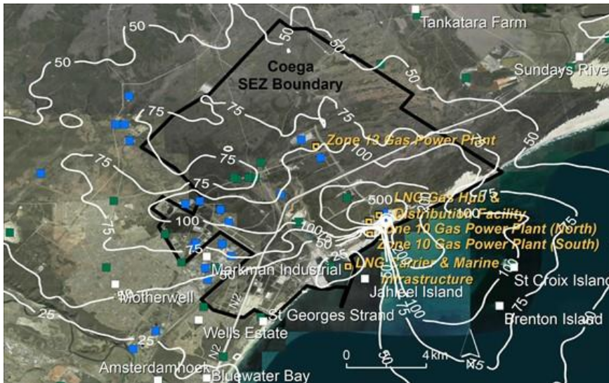
Figure 23: Predicted 1-hour CO concentrations in \mu\text{g}/\text{m}^3 for Scenario 1 the Land-based LNG Terminal and Infrastructure Project (top left), Scenario 2 the Land-based LNG Terminal and Infrastructure Project with baseline (top right), Scenario 3 the 3 000 MW Coega G2P Project (bottom left) and Scenario 4 the 3 000 MW Coega G2P Project and baseline (bottom right)
