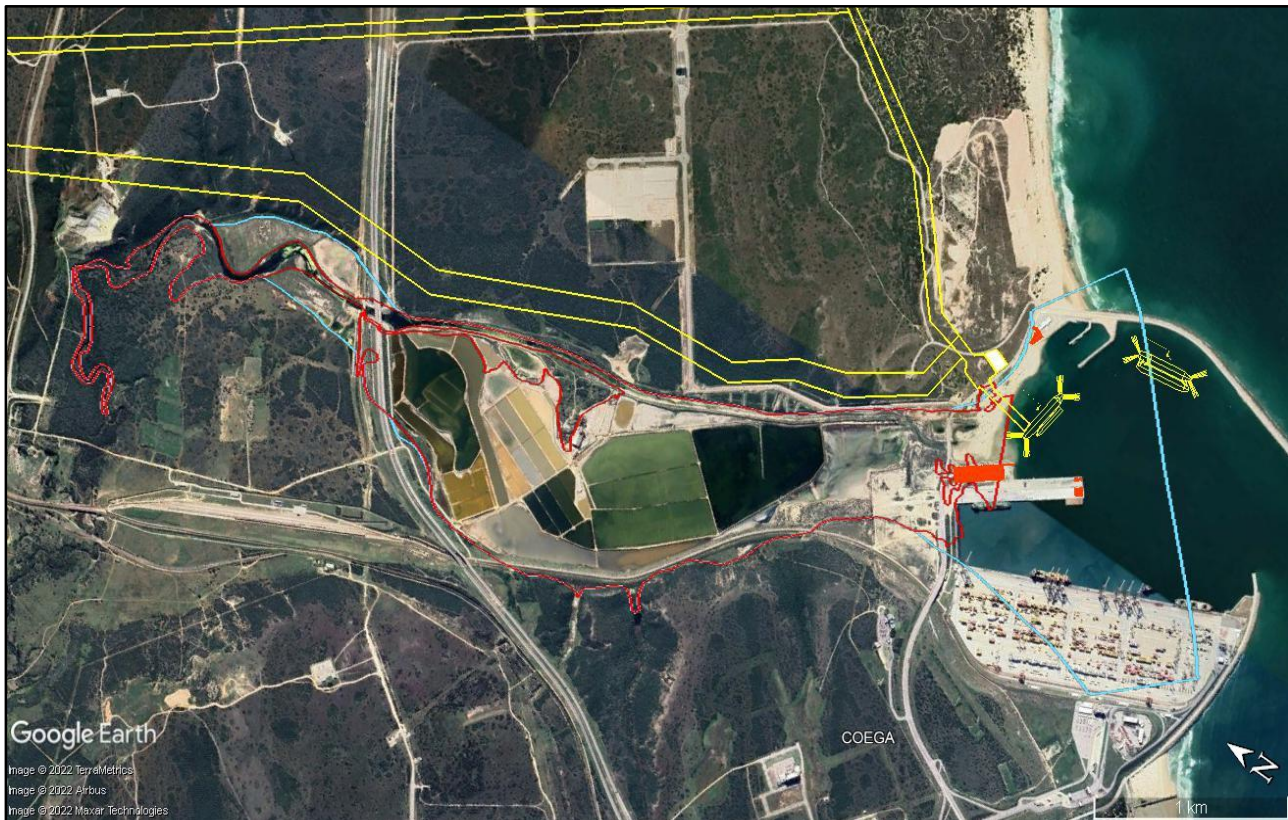
Figure 6-16: Geographical boundaries of the Coega estuarine functional zone as delineated by the 5m topographical contour in red, and the 10m topographical contour and marine extension in blue (Image source: Google Earth, 2021). Components of the Gas to Power project indicated in yellow (vessels, pipelines and transmission line corridors) and orange (contractor facilities)
