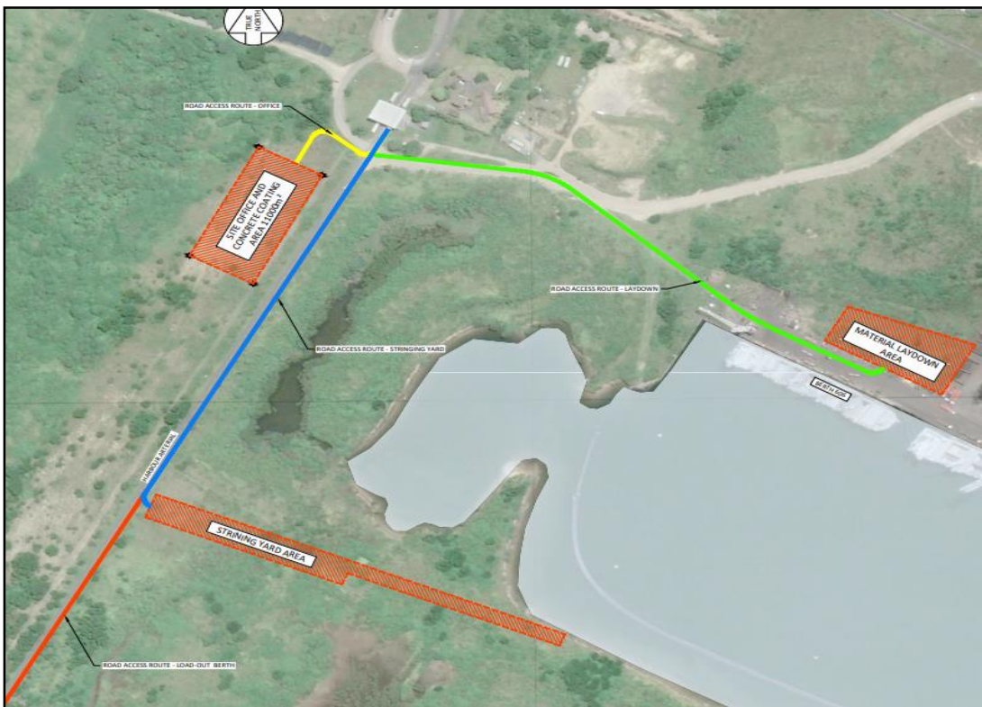
Figure 3-8: Proposed locations for the temporary construction facilities
