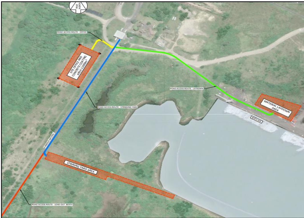
Figure 2-11: Access roads to temporary construction facilities – existing roads (blue and green) and proposed road (yellow)
