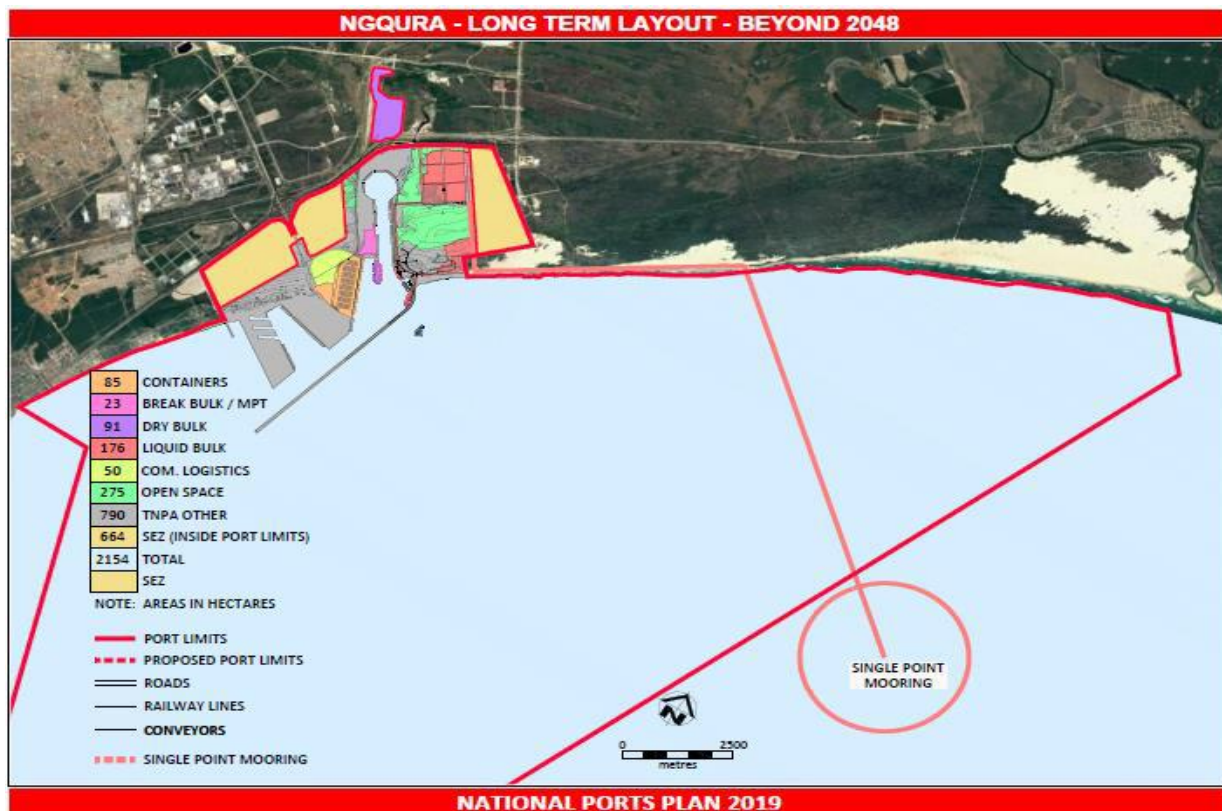
Figure 6-8: Port of Ngqura long-term layout (incl. the new SPM).
